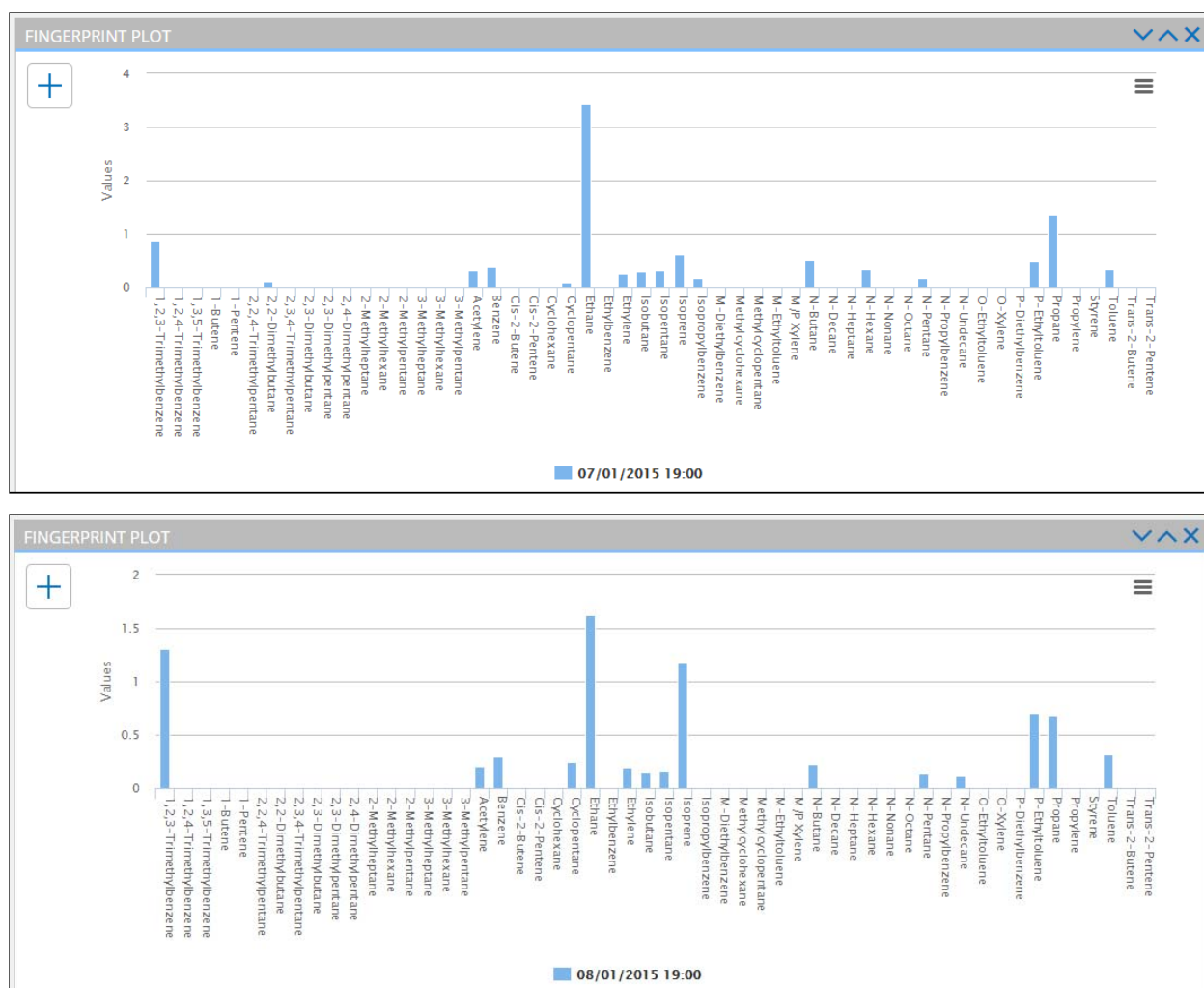
Figure 10-4. Fingerprint Plots of PAMS Target VOC Analytes
