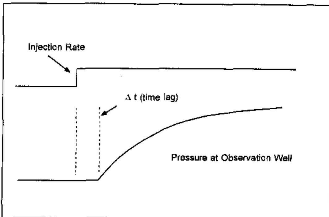
The dashed line in Graph S3-G2 shows a time lag from when injection starts in the active well and the observed pressure increase in the observation well. This time lag is a function of the rock and fluid properties between the wells. The term that defines the time lag is known as the diffusivity constant<sup>1</sup> and is defined as
