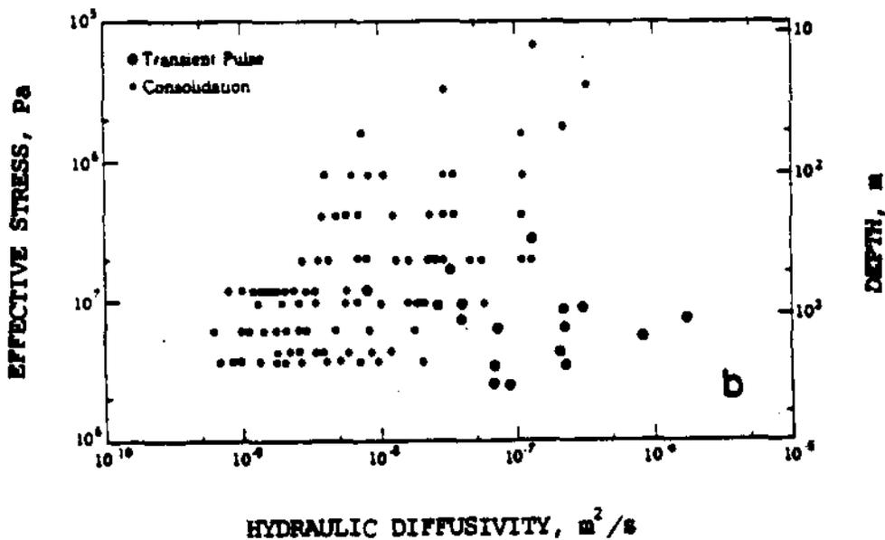
Hydraulic properties of the Pierre Shale derived from a steady flow test and transient hydraulic and mechanical tests. The transient hydraulic test methodology used was that described by Reich et al. (1981) and Nouril et al. (1981); the transient mechanical tests were step load consolidation (e.g., Scott, 1963). The data are plotted against effective stress and as equivalent depth in meters using the convention that effective stress increases at approximately  $1.3 \times 10^4$  Pa/m.
