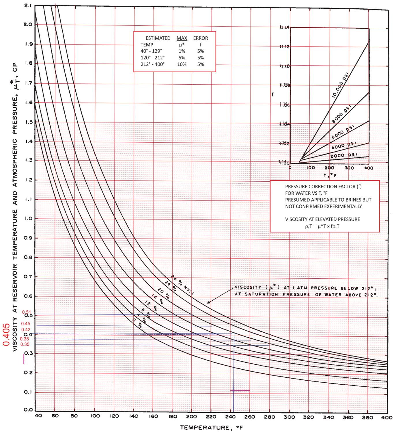
Fig. D.35 Water viscosity at various salinities and temperatures After Mathews and Russell, data of Chesnut
