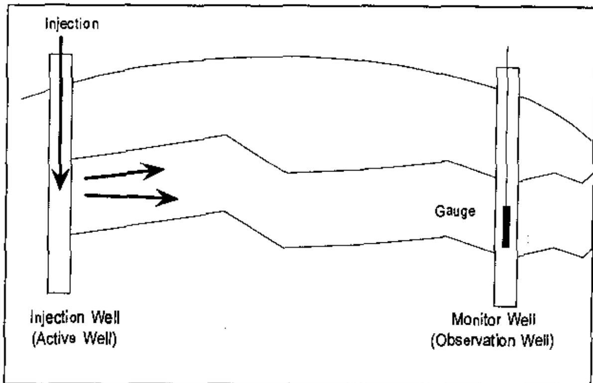
Graph S3-G2 on the next page shows the theoretical pressure response created in the observation well during injection into the active well. Pressure will increase exponentially, and proportionally to the distance and reservoir properties between the wells. The magnitude of the pressure increase is governed by the rate, the distance between wells, and the average transmissibility between wells.
