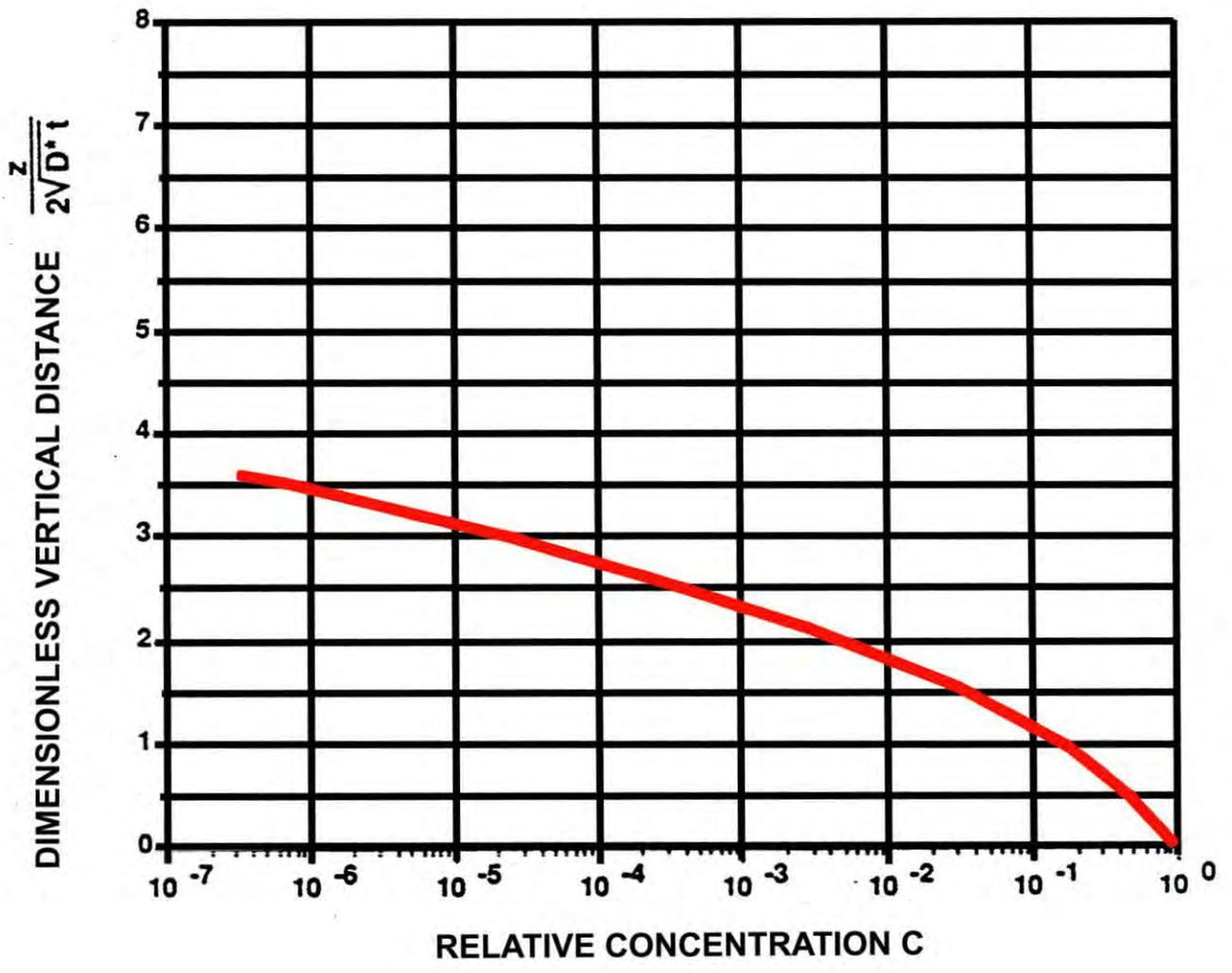
Figure 3: Predicted Concentration Profile (Logarithmic Plot).
