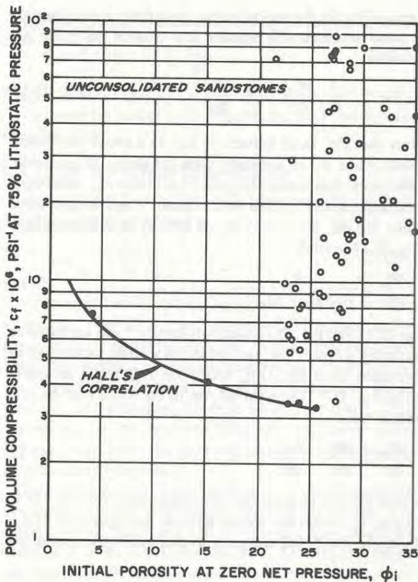
Fig. D.12 Pore-volume compressibility at 75-percent lithostatic pressure vs initial sample porosity for unconsolidated sandstones. After Newman.<sup>9</sup>
