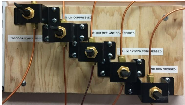
Open: switch is 180°, Closed: switch is 90°
