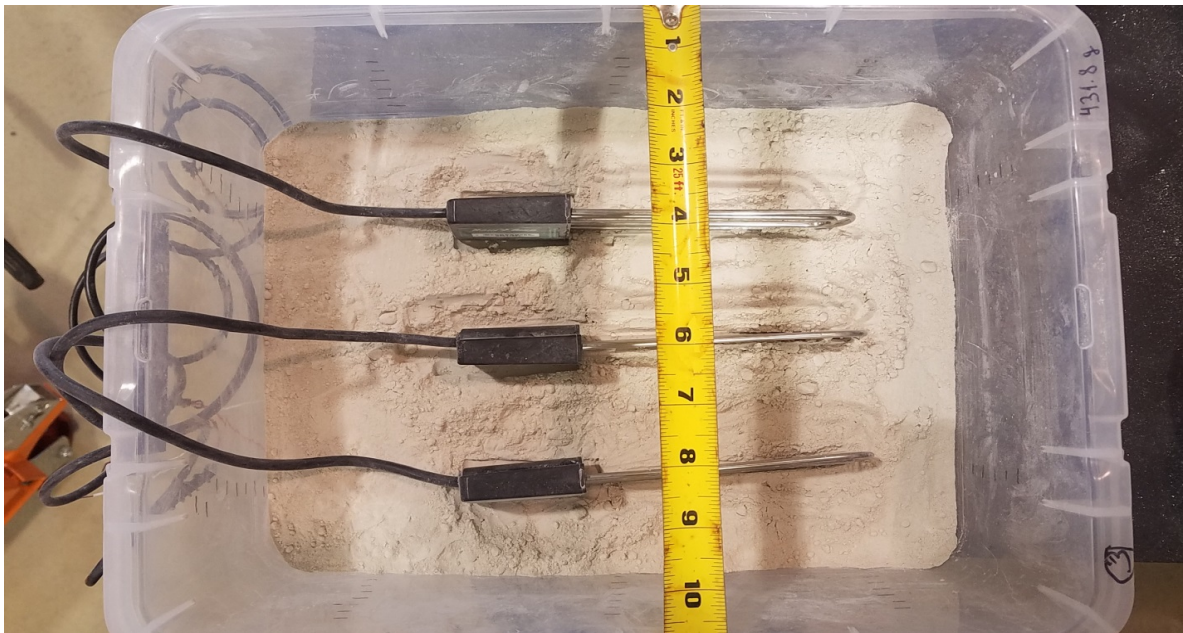
Figure 4. Installation of sensor mechanisms during packing (credit Bernard Cardenas UF/IFAS)
