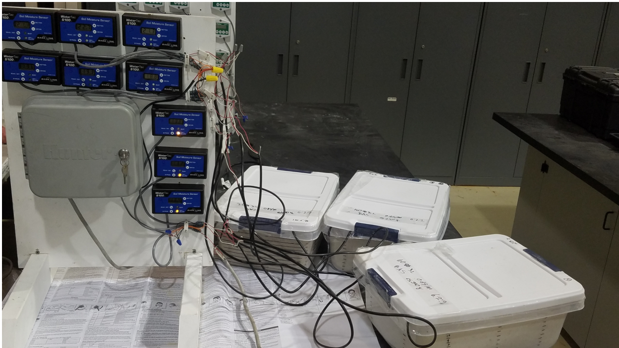
Figure 6. Testing of SMS controllers powered by an irrigation controller (credit Bernard Cardenas UF/IFAS)
