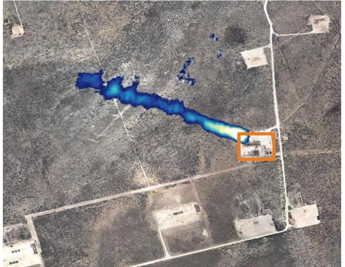
Kairos sensor pods deploy on light aircraft, imaging, quantifying, and source-attributing methane from 3,000 feet, covering 100-150 square miles per day.
