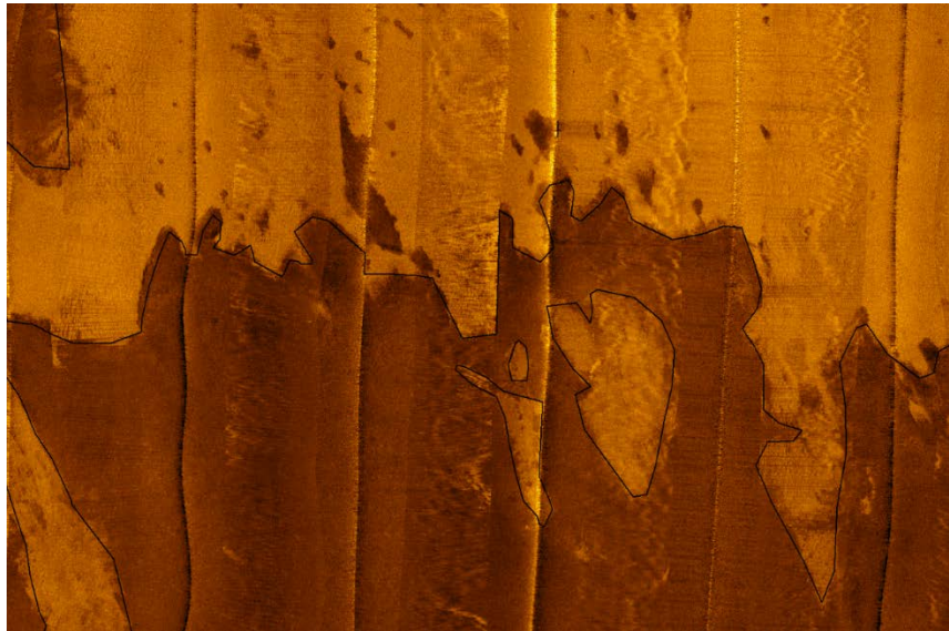
Figure 1: Example of the two identified surface sediment types. Texture 1: high backscatter (upper portion of image). Texture 2: medium intensity backscatter (lower part of image).
