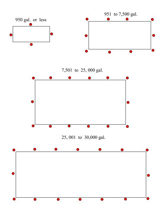
• Sampling points are located as near to tanks as possible.
