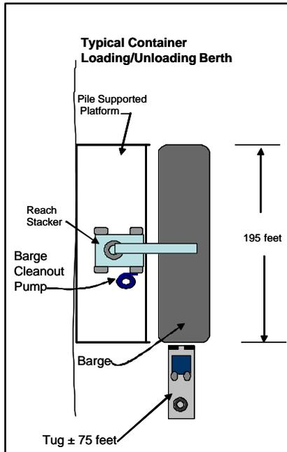
A mobile “reach stacker” will be required for Alternative 2, where processed material is loaded into containers and transported to a transloading facility by barge. A separate berth located near shore will be required for this operation.
