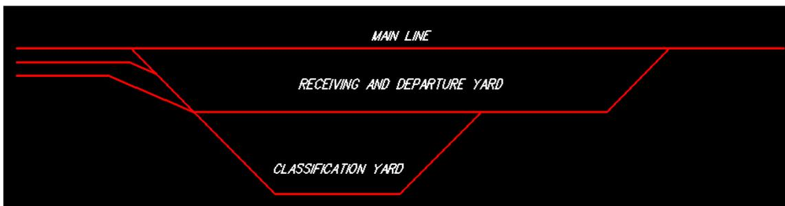
Figure 9-A-1 – Typical Flat Switching Yard
