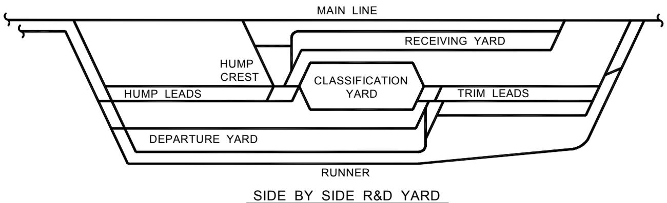
**Figure 9-A-3 – Side-By-Side Receiving and Departure Yard**
