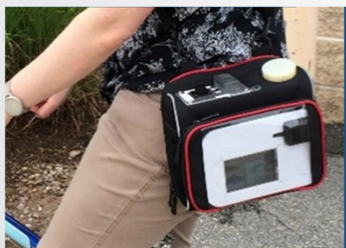
Custom built AirMapper (PM 2.5 , CO 2 , GPS, noise, T, RH)
