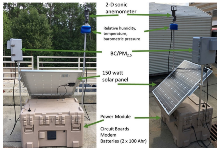
Custom built P-Pod (BC, PM 2.5 , WS/WD, T, RH, P)
