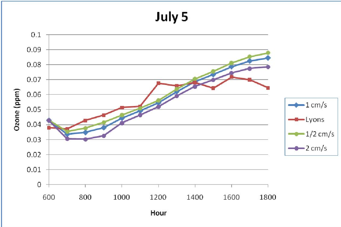
**Figure 6.2:** Sensitivity of predicted ozone concentrations on July 5 to changes in ozone deposition rates and comparison of to observed concentrations at Lyons, CO
