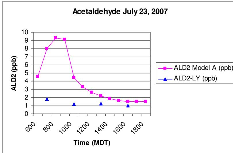
**Figure 6.7:** Comparison of OZIPR predictions and observed acetaldehyde concentrations at Lyons, CO
