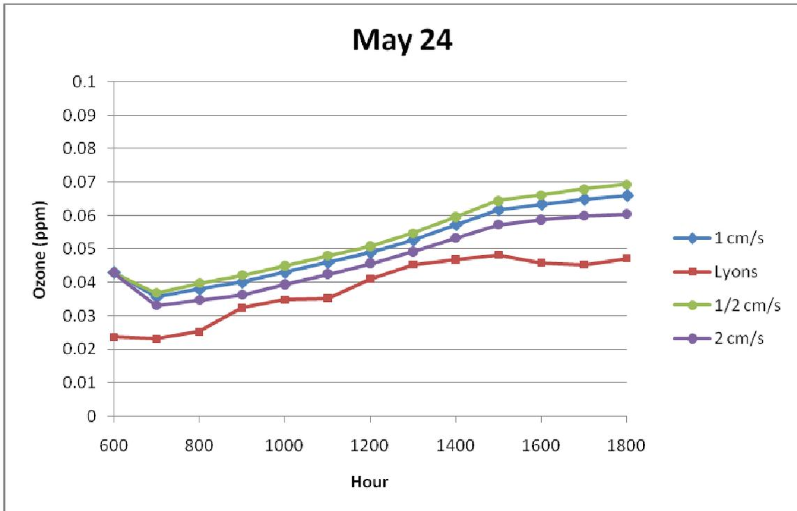
**Figure 6.3:** Sensitivity of predicted ozone concentrations on May 24 to changes in ozone deposition rates and comparison of to observed concentrations at Lyons, CO
