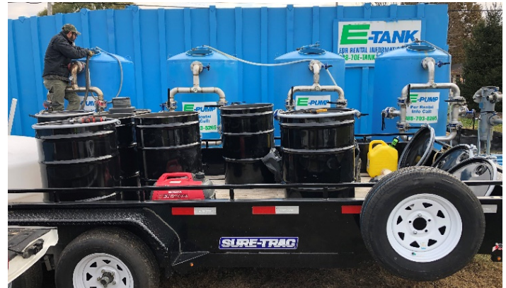
Photo #2: Transferring clay filtering media from filter pot to drums using a drum vacuum
