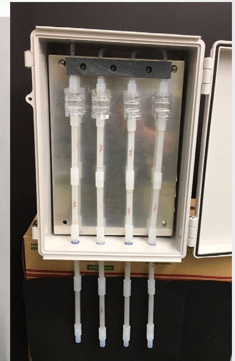
4 denuders in series X 4 sets per sample box
