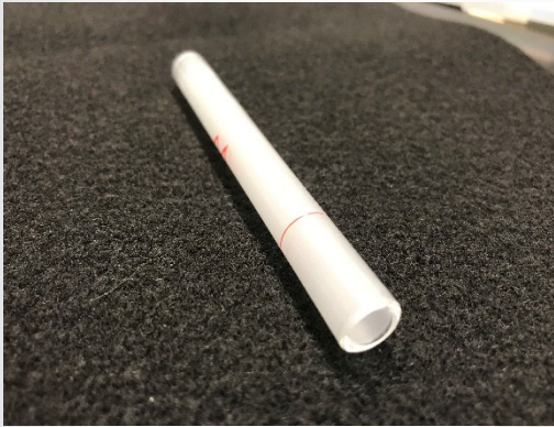
Glass denuder Single bore 10 cm length
