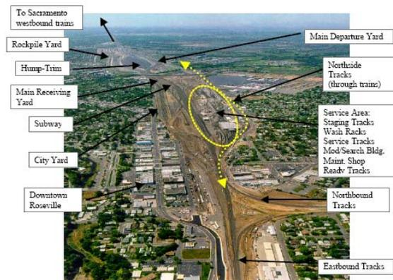
Figure 2. Operational Layout of Railyard
