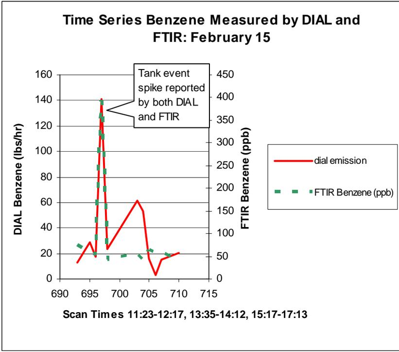
**Figure 4.1l Time Series Benzene Measured by DIAL and FTIR: February 15**
