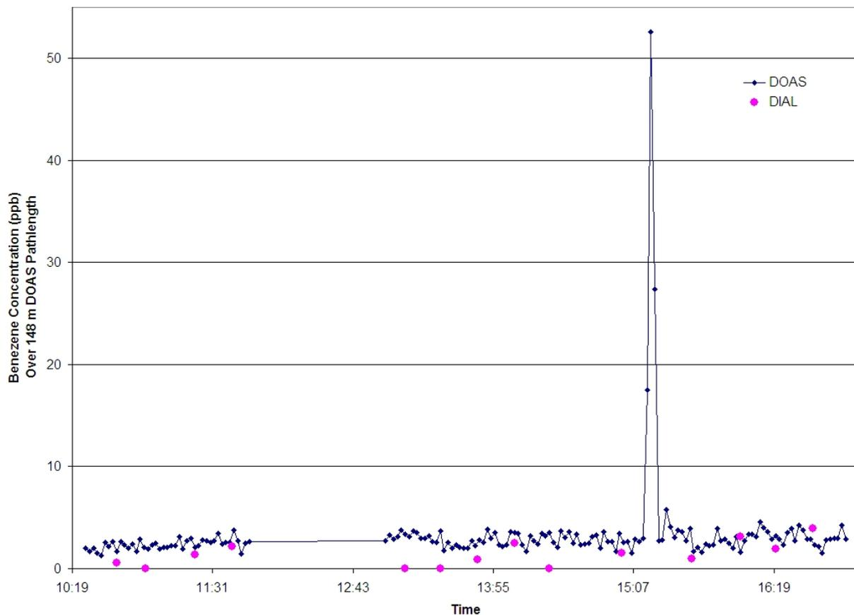
**Figure 5.4 DIAL and DOAS measurements comparison on the 9<sup>th</sup> of February.**
