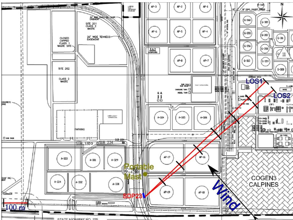
Figure 3.1 Measurement configuration for location SDP23 on 8<sup>th</sup> of February.
