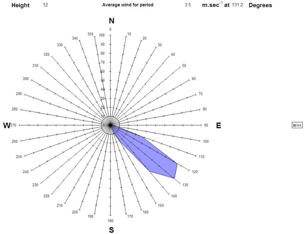
**Figure A3.12 Wind rose for 23<sup>rd</sup> January during measurements from SDP11, 10:57 - 17:06**
