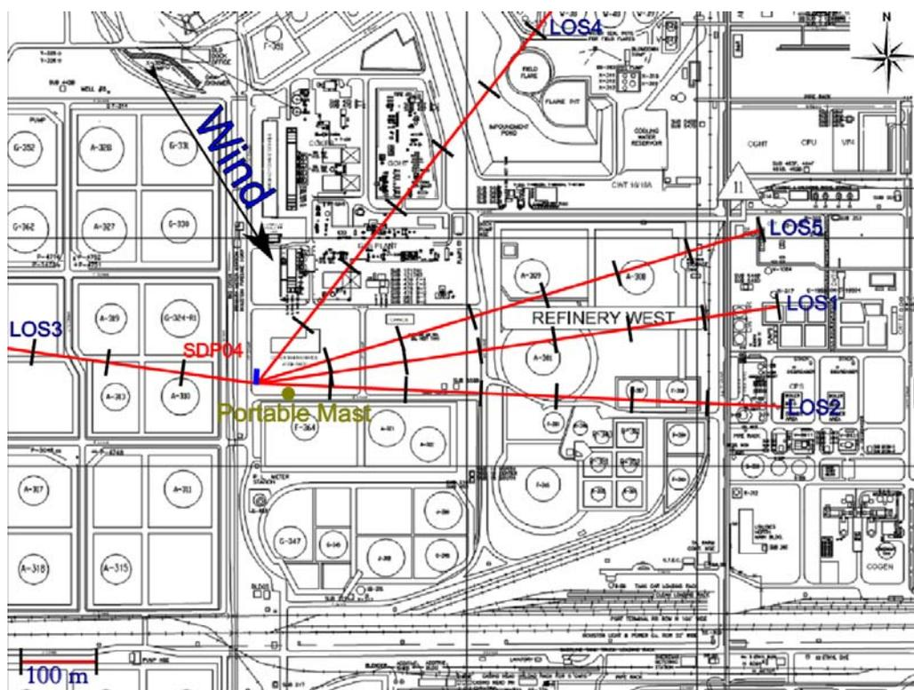
Figure 2.4 Measurement configuration for location SDP04 on 16<sup>th</sup> of January.
