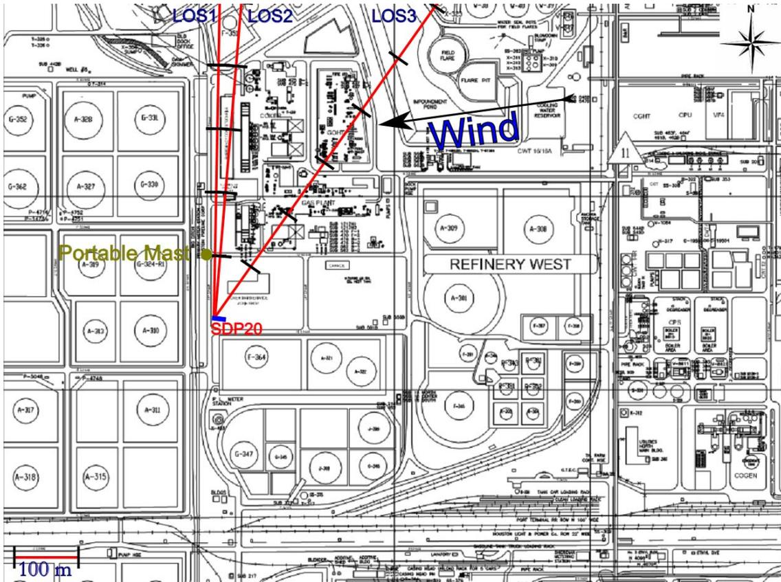
Figure 2.21 Measurement configuration for location SDP20 on 4<sup>th</sup> of February.
