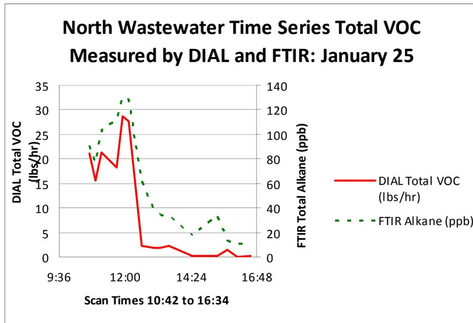
**Figure 4.1a North Wastewater Time Series Total VOC Measured by DIAL and FTIR: January 25**
