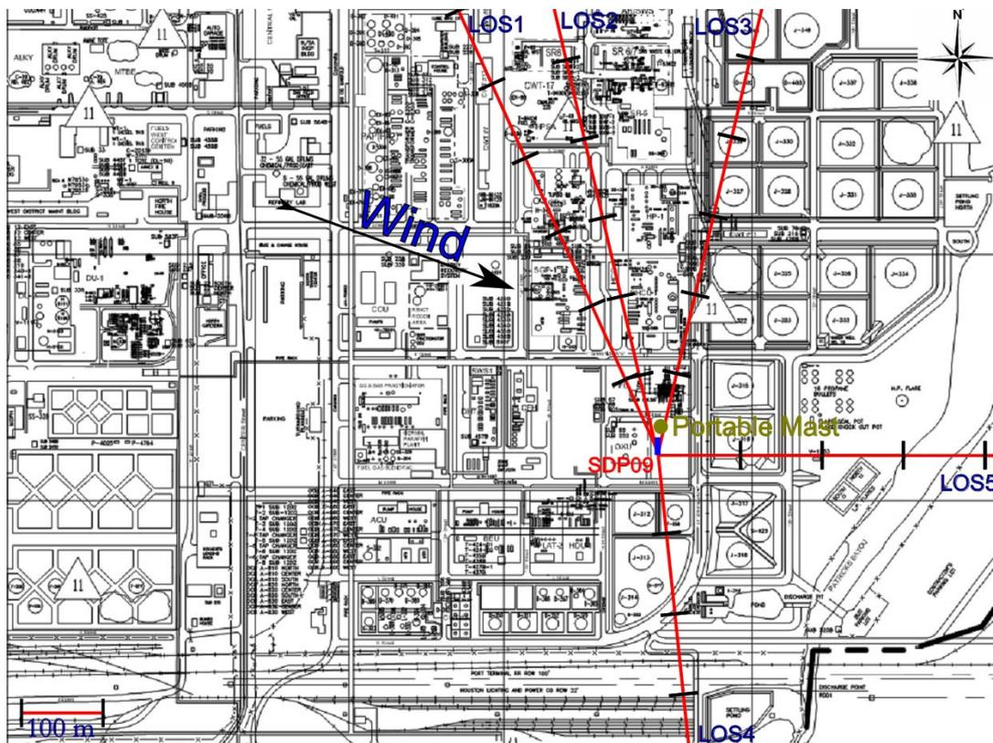
Figure 2.9 Measurement configuration for location SDP09 on 21<sup>st</sup> of January.
