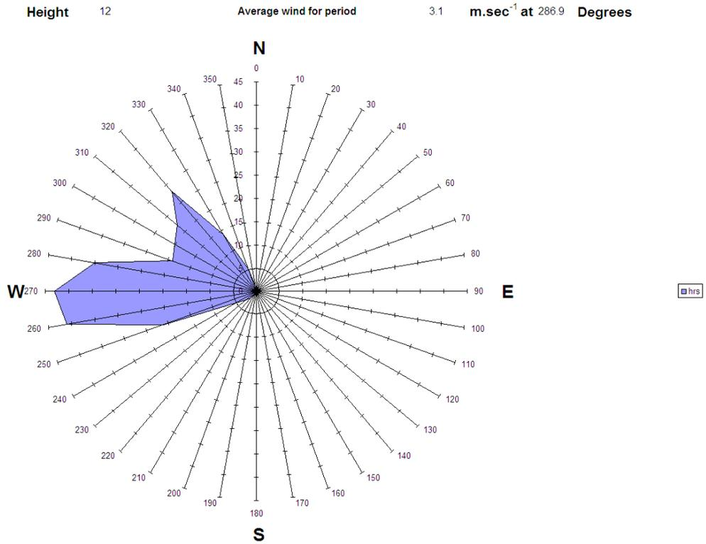
**Figure A3.10 Wind rose for 21<sup>st</sup> January during measurements from SDP9, 11:57 - 16:55**
