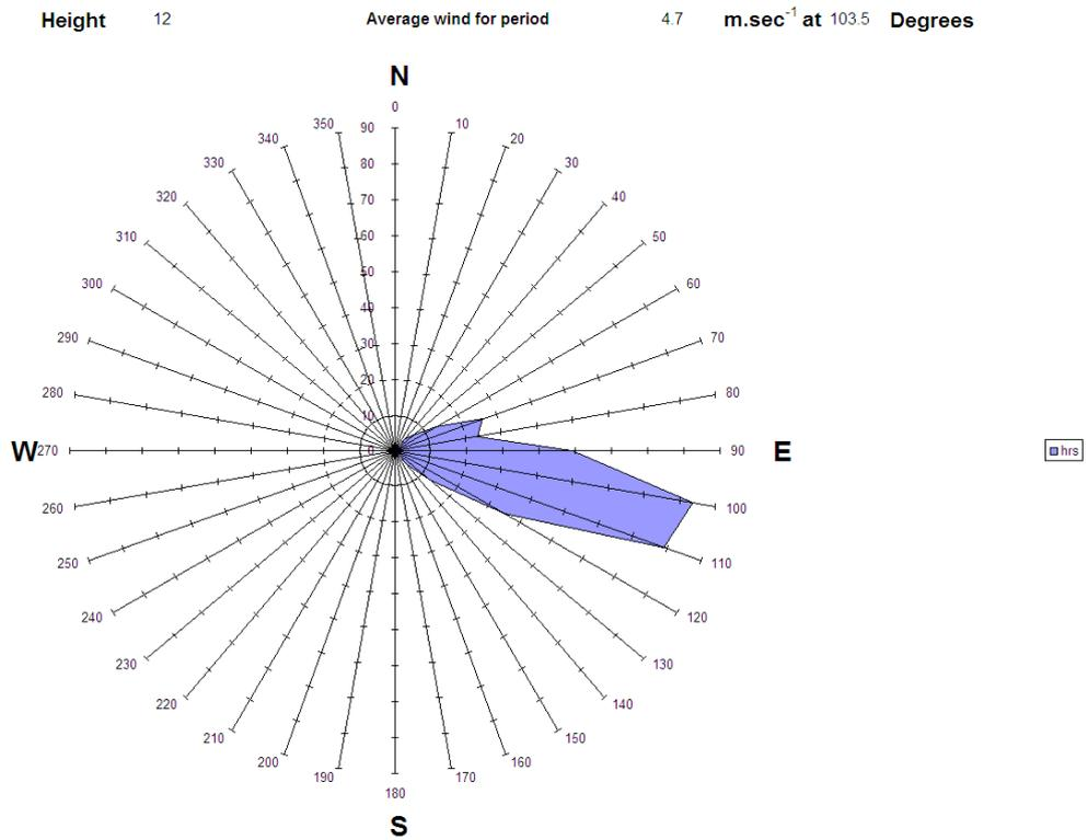
**Figure A3.21 Wind rose for 3<sup>rd</sup> February during measurements from SDP19, 10:30 - 16:54**
