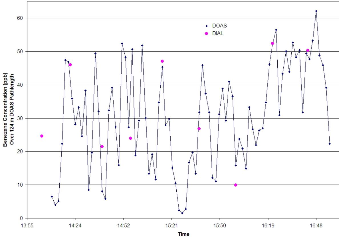
**Figure 5.3 DIAL and DOAS measurements comparison on the 10<sup>th</sup> of February from 14:00.**
