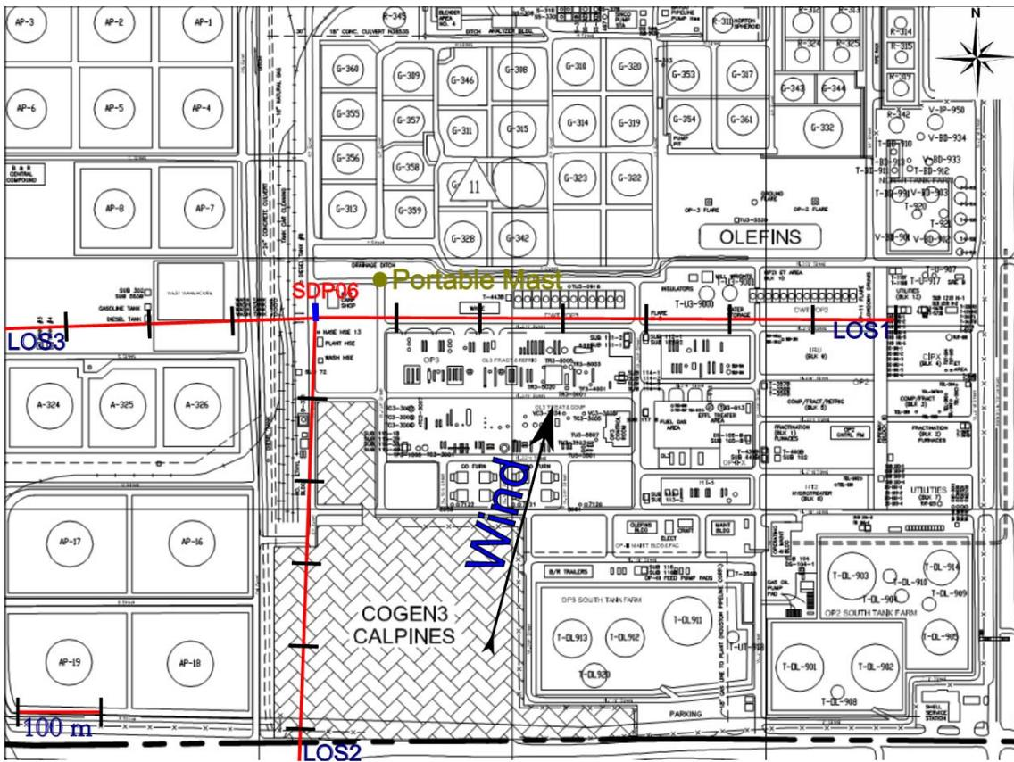
Figure 2.6 Measurement configuration for location SDP06 on 19<sup>th</sup> of January.
