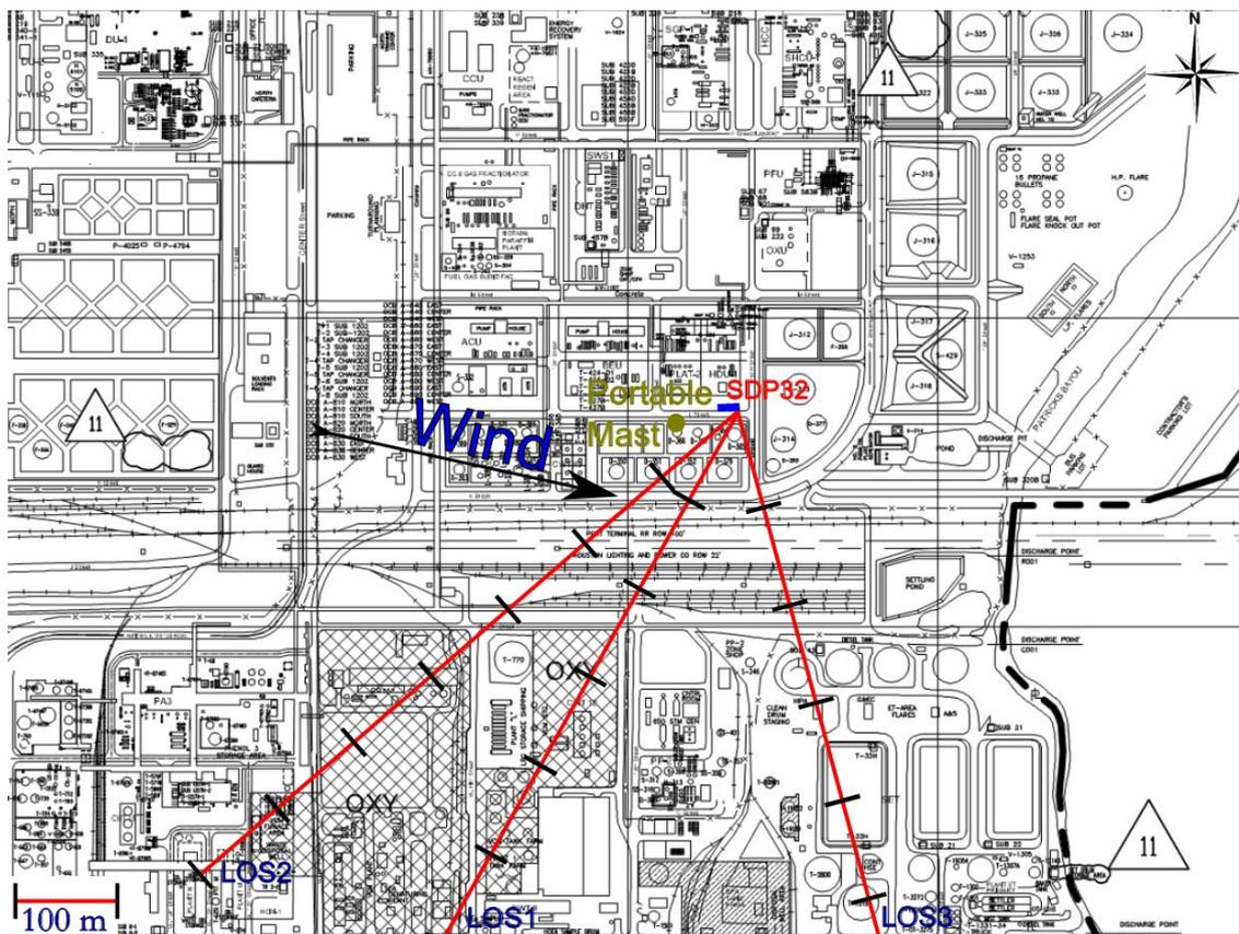
Figure 3.11 Measurement configuration for location SDP32 on 22<sup>nd</sup> of March.
