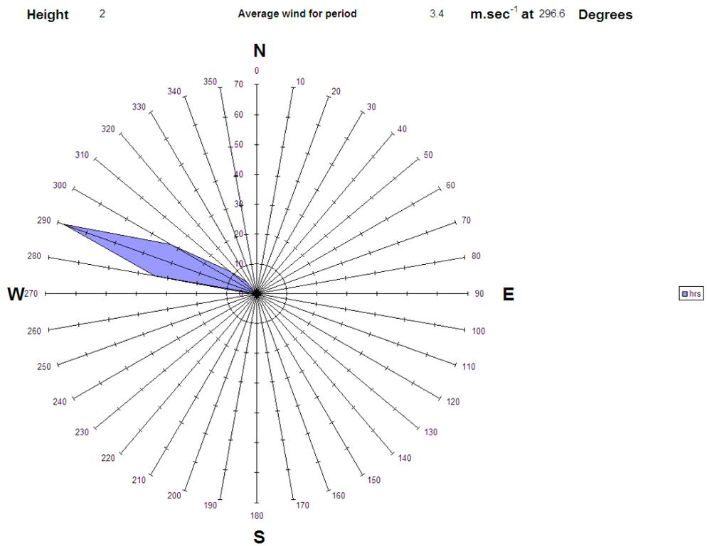
**Figure A3.23 Wind rose for 5<sup>th</sup> February during measurements from SDP21, 10:50 - 14:11**
