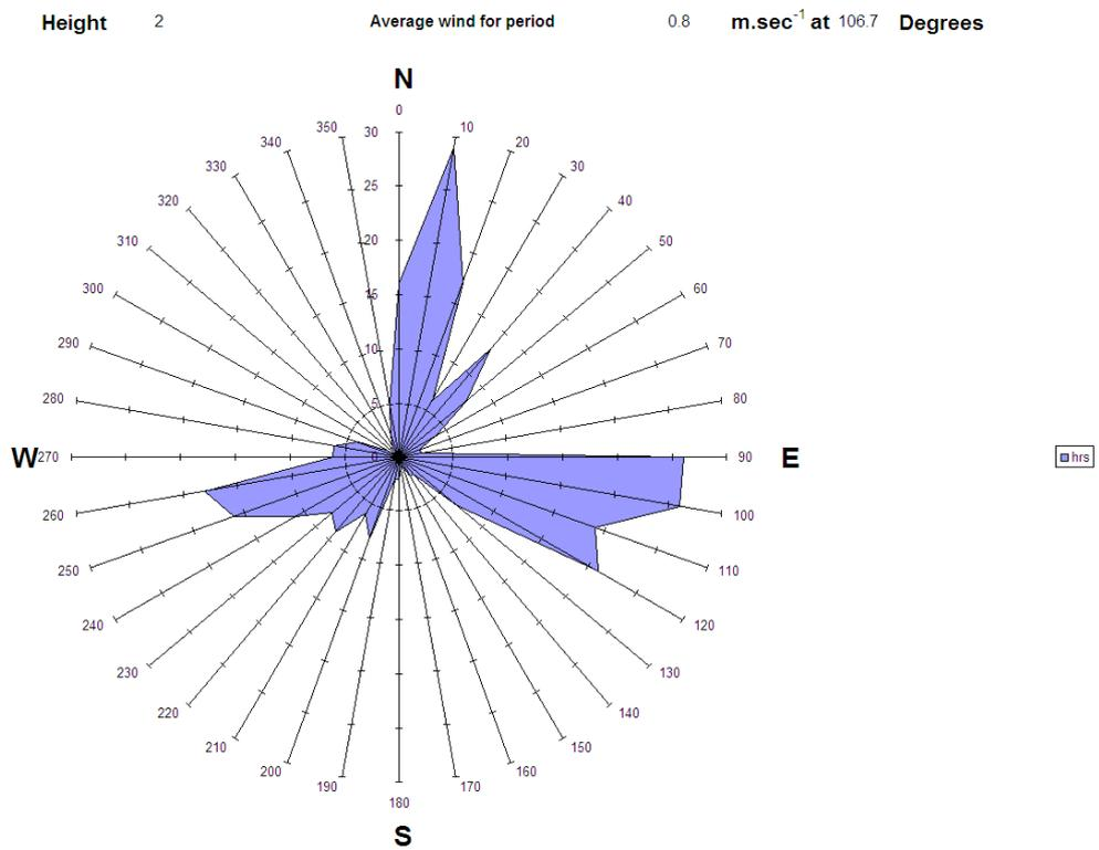
**Figure A3.13 Wind rose for 25<sup>th</sup> January during measurements from SDP12, 10:42 - 17:01**
