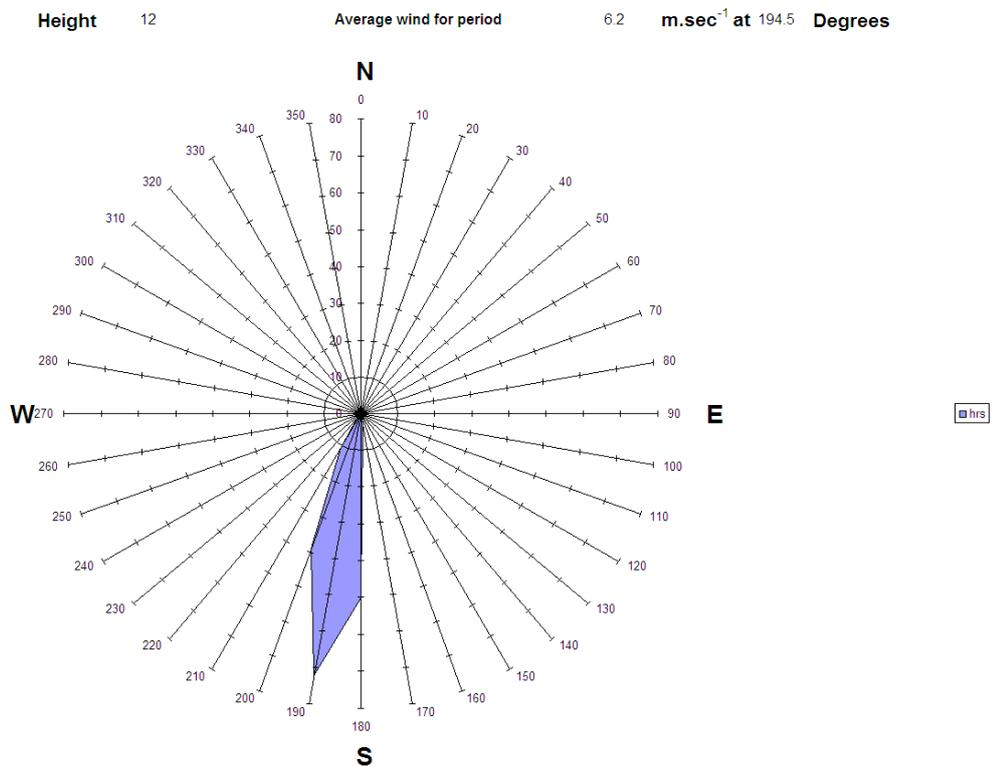
Figure A3.7 Wind rose for 19<sup>th</sup> January during measurements from SDP6, 10:27 - 14:18
