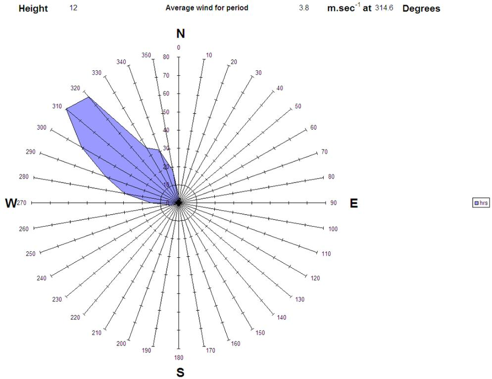
Figure A3.32 Wind rose for 15<sup>th</sup> February during measurements from SDP28, 10:18 - 17:13
