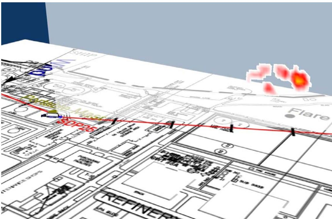
Figure 3.3b2 Visualisation of emission rate measured for Scan 574 representing LOS2.
