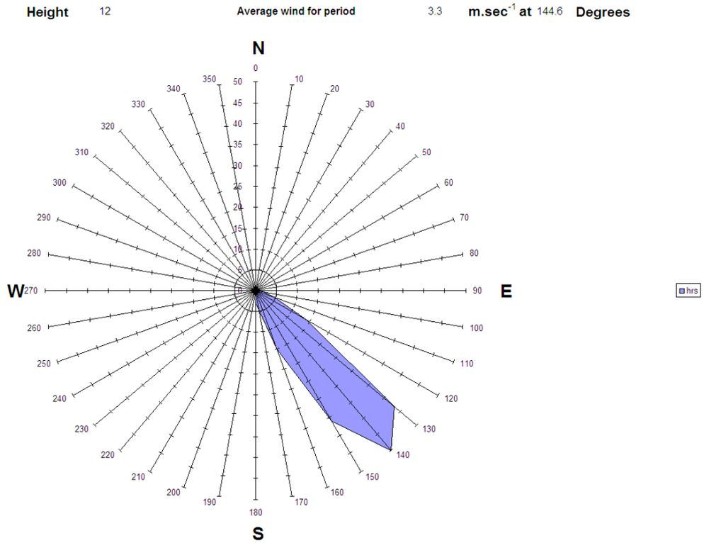
Figure A3.26 Wind rose for 8<sup>th</sup> February during measurements from SDP24, 14:15 - 17:23
