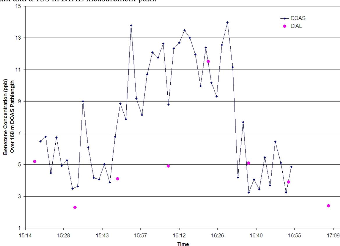
**Figure 5.1 DIAL and DOAS measurements comparison on the 8<sup>th</sup> of February.**
