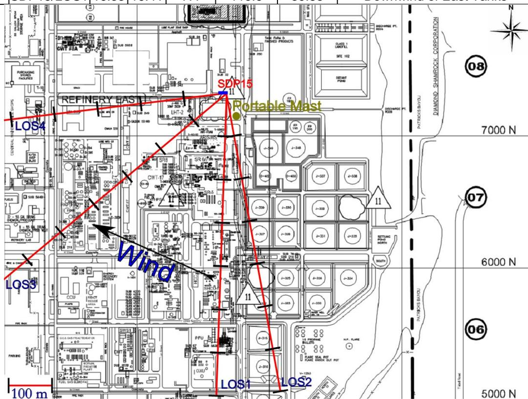
Figure 2.15 Measurement configuration for location SDP15 on 28<sup>th</sup> of January.
