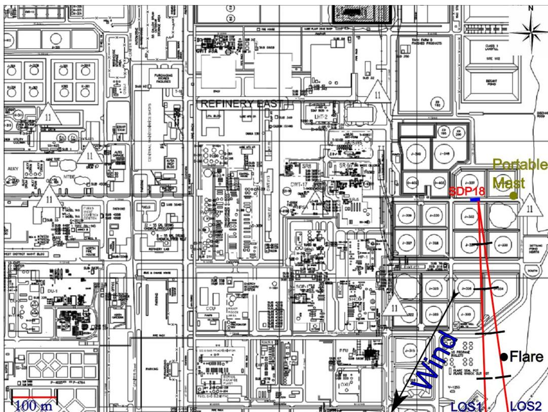
Figure 2.19 Measurement configuration for location SDP18 on 2<sup>nd</sup> of February.
