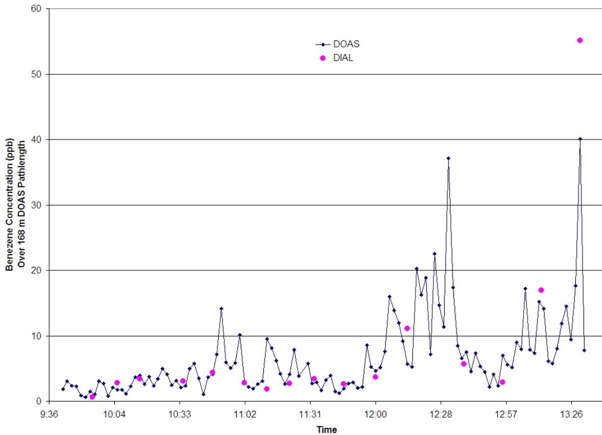
**Figure 5.2 DIAL and DOAS measurements comparison on the 10<sup>th</sup> of February until 13:30.**
