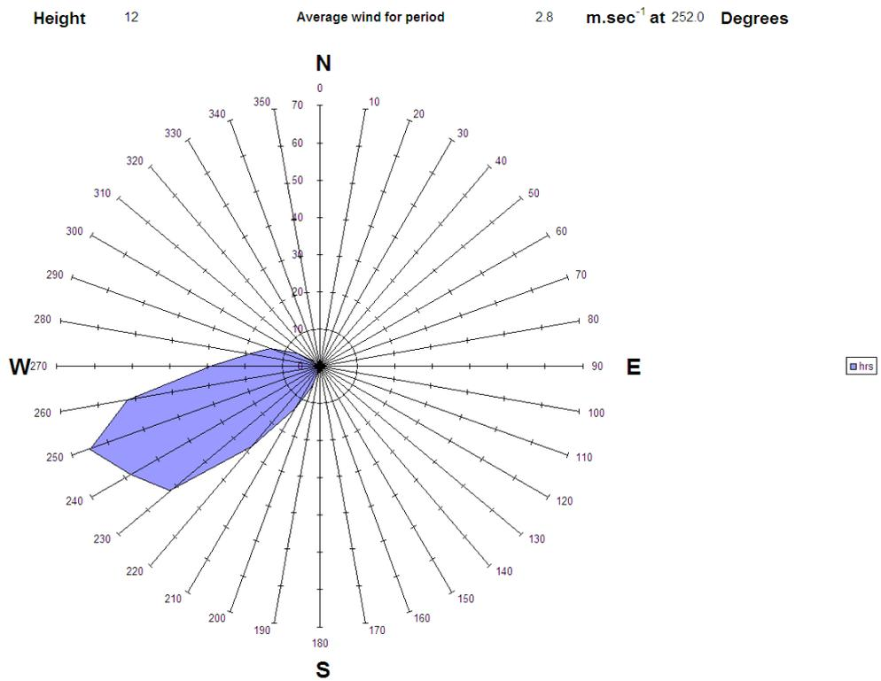
Figure A3.31 Wind rose for 13<sup>th</sup> February during measurements from SDP29, 10:53 - 16:42
