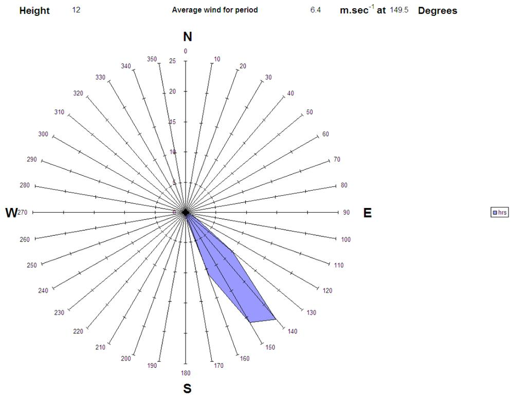
**Figure A3.25 Wind rose for 8<sup>th</sup> February during measurements from SDP23, 10:55 - 12:07**
