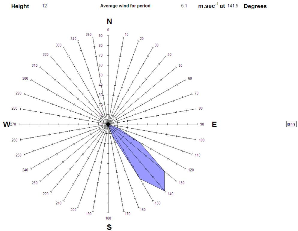
**Figure A3.11 Wind rose for 22<sup>nd</sup> January during measurements from SDP10, 12:07 - 17:30**
