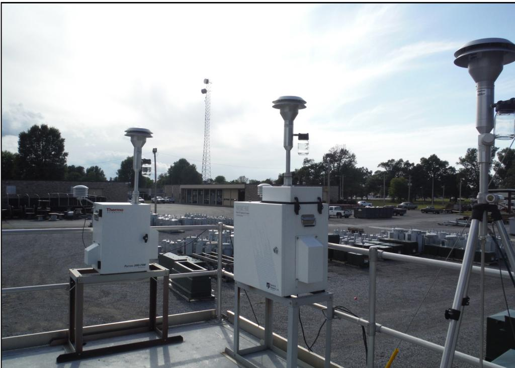
**Figure 2: Picture of the intermittent  $PM_{2.5}$  and  $PM_{10}$  samplers, as well as the inlet of the  $PM_{2.5}$  TEOM, on the roof of the Jackson Purchase RECC shelter on October 6, 2014.**
