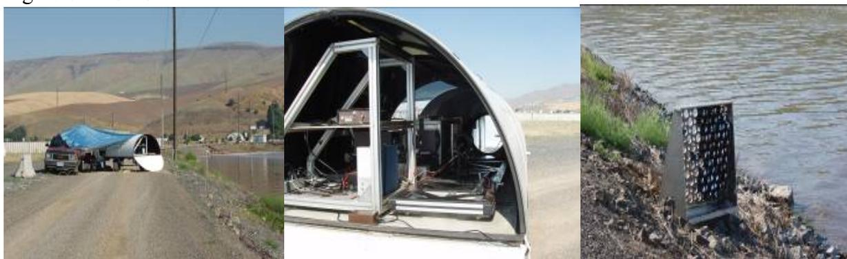
A Proton Transfer Reaction Mass Spectrometer (PTR-MS) mobile laboratory system (Figure 7) was utilized for a few days for establishing a correlation of three independent measurement techniques for formaldehyde concentrations. The PTR-MS instrument was not part of the original proposal but was available at an opportune time for the experiments.
