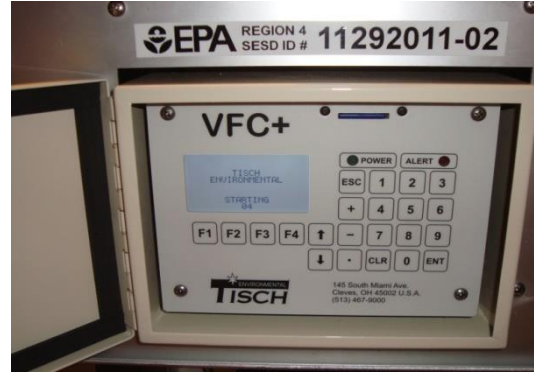
Figure 5-11. Tisch Sampler's Main Menu Screen
