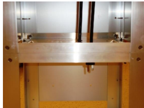
Figure 5-4. Completely Aligned Sampler and Leg/Base Assembly for the Tisch Sampler
