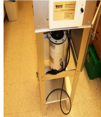
Figure 5-8. Electrical Connection of the VFC to the Tisch Sampler Main Unit
