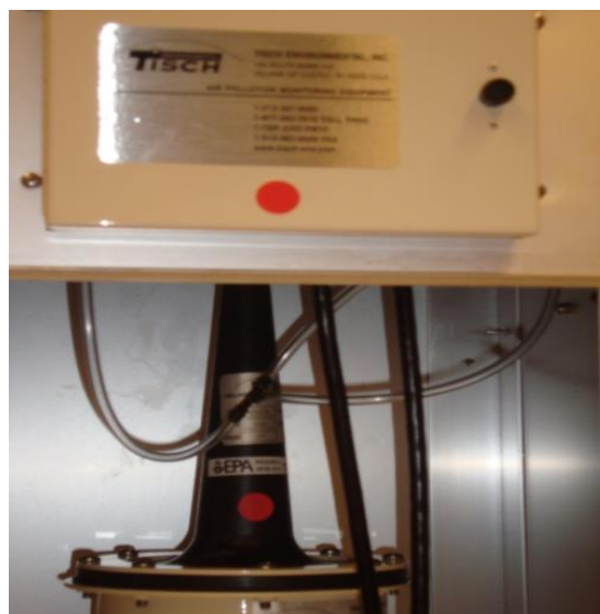
Figure 5-6. Unique Labels for the Tisch Sampler's VFC and VFC+ Controller Box/Main Unit
