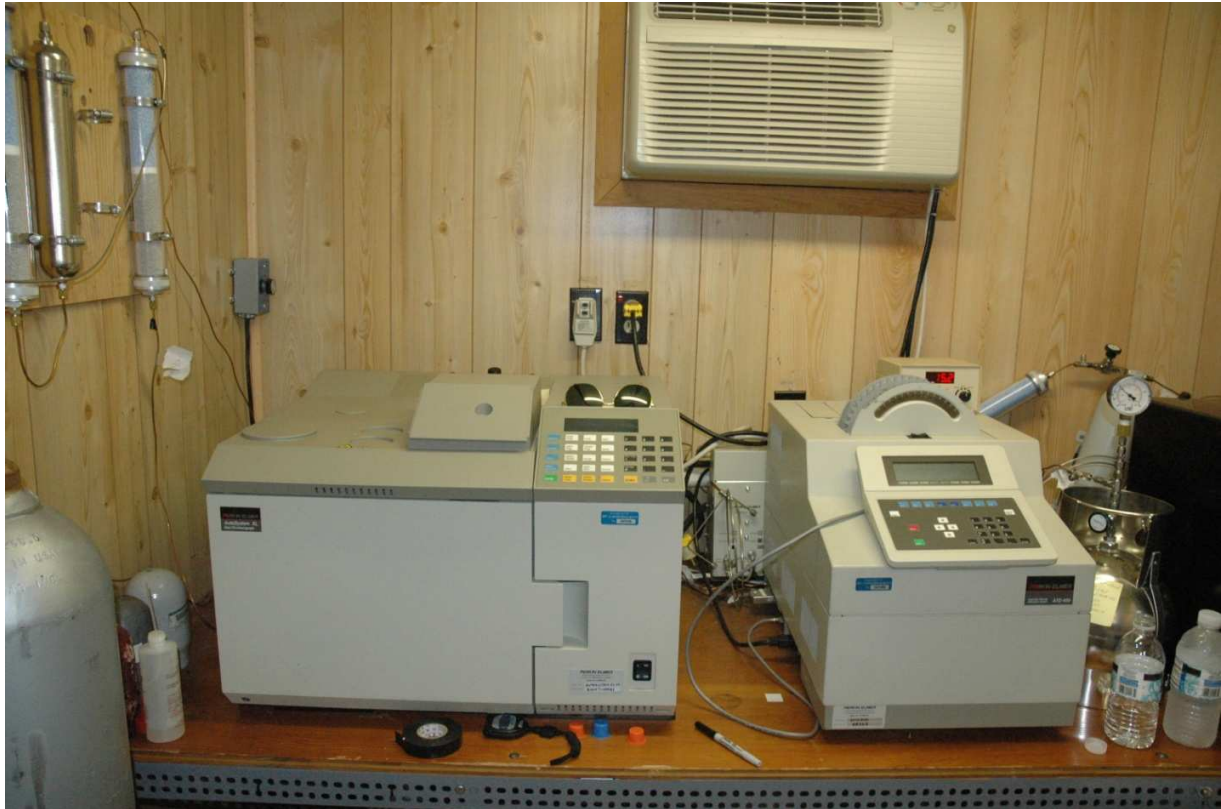
Figure 3.8.1 Automated GC in operation at the Henrico County site
