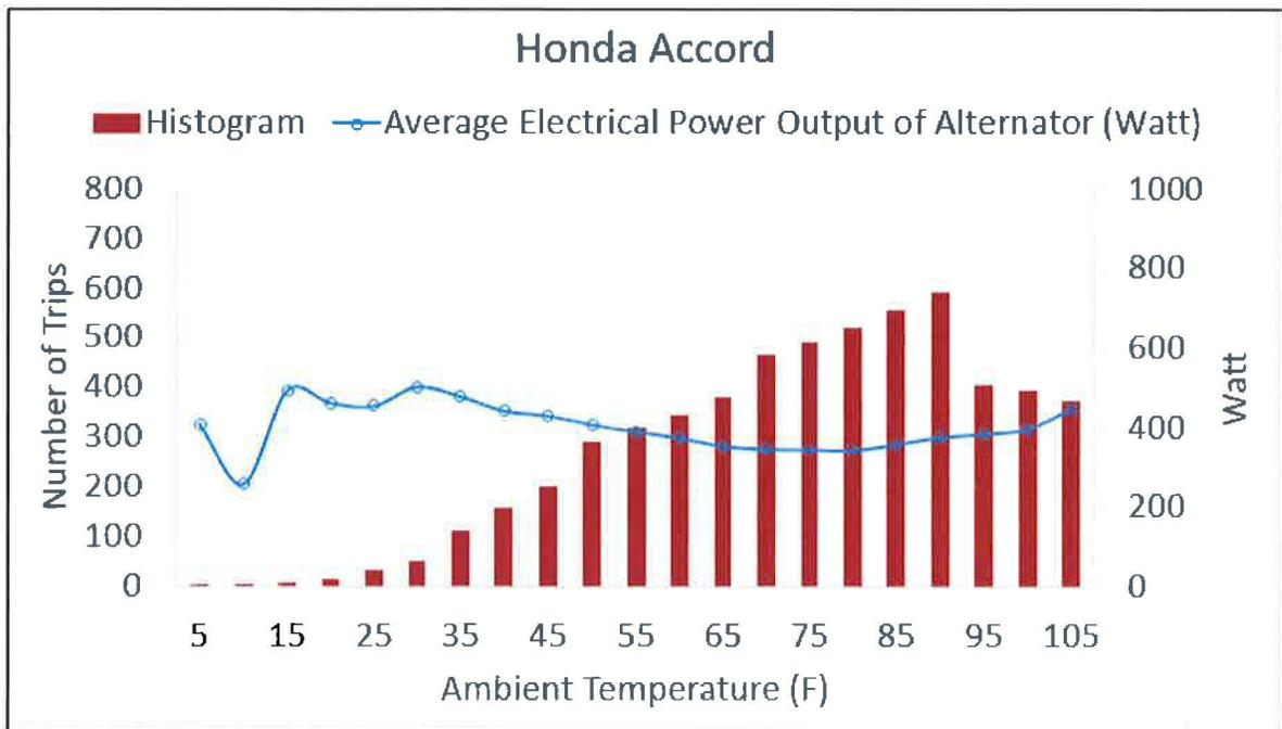
**Fig. 1-1. On-road electrical power output of alternator (2010MY Honda Accord)**
