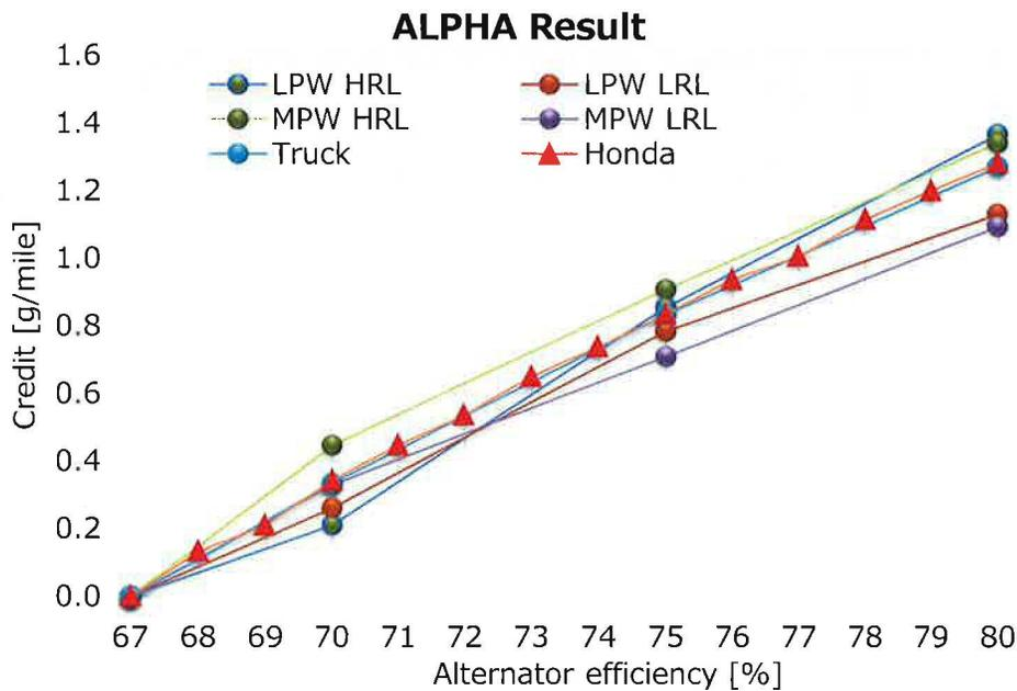
Fig. 2. Comparison of proposed credit (Honda) and simulation by ALPHA
