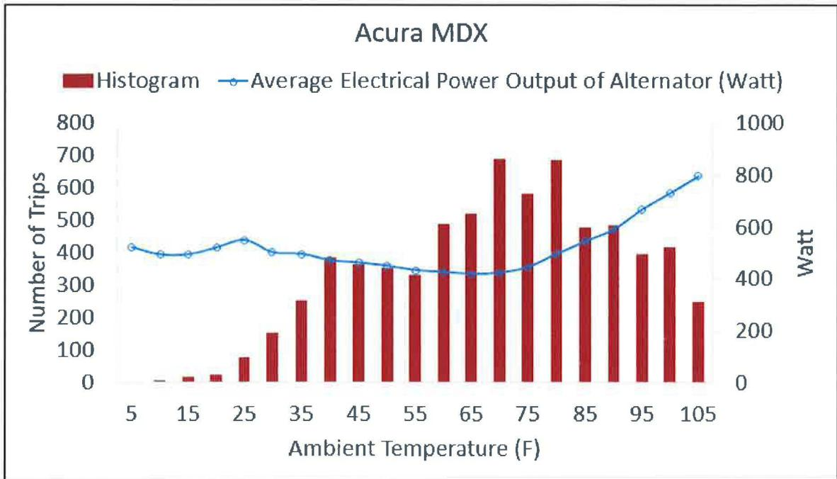
Fig. 1-2. On-road electrical power output of alternator (2010MY Acura MDX)
