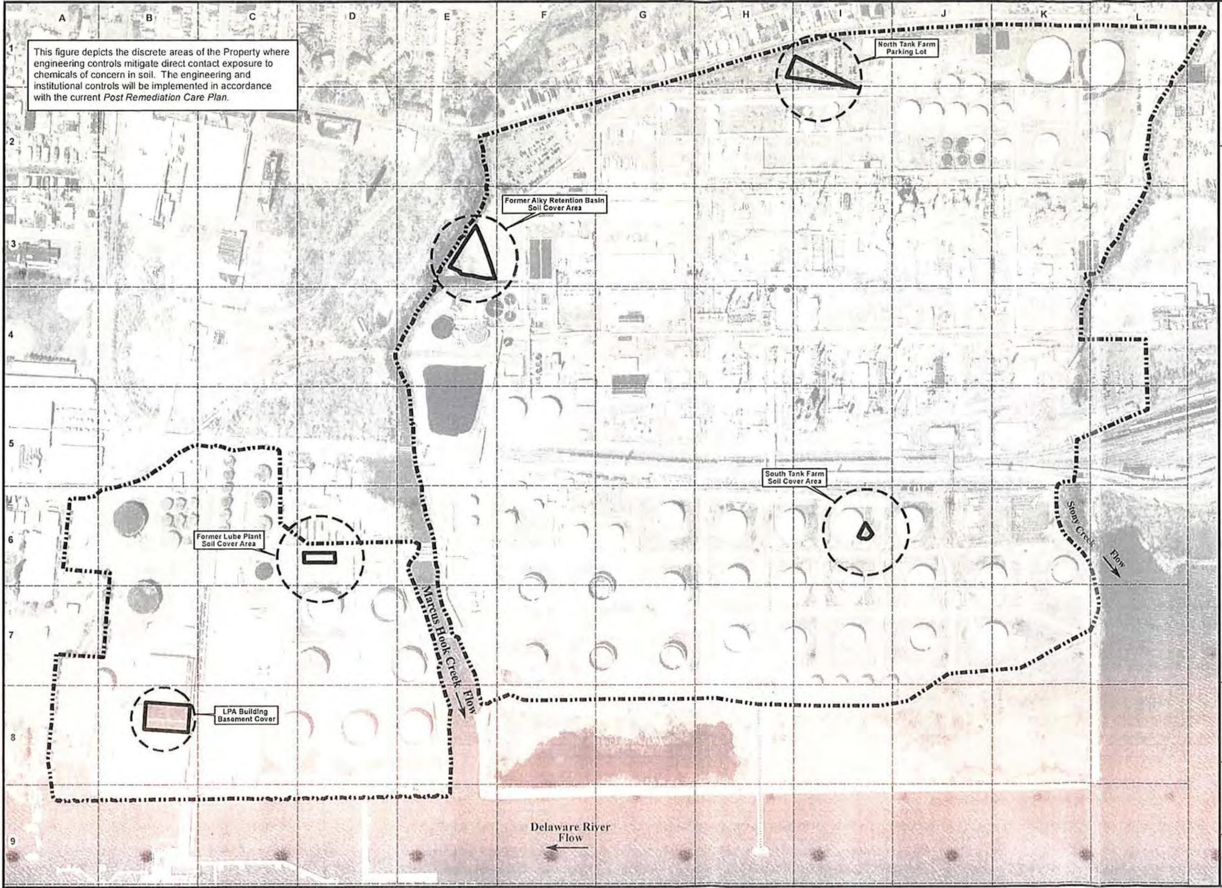
This figure depicts the discrete areas of the Property where engineering controls mitigate direct contact exposure to chemicals of concern in soil. The engineering and institutional controls will be implemented in accordance with the current *Post Remediation Care Plan*.
