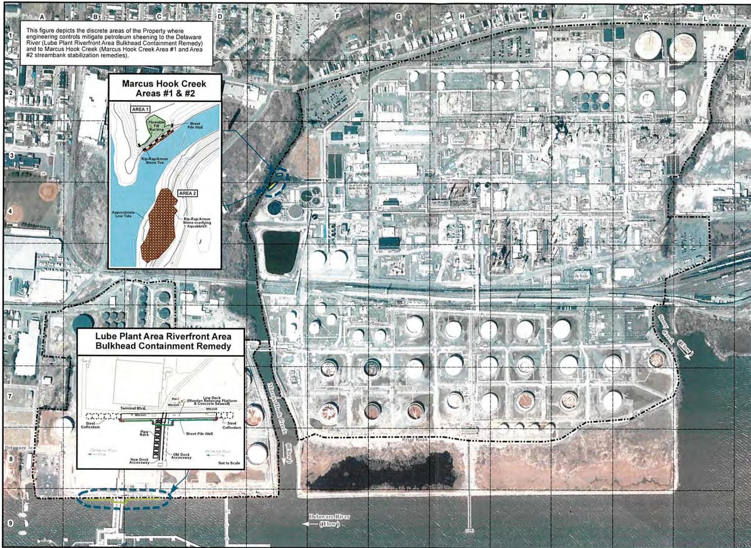
This figure depicts the discrete areas of the Property where engineering controls mitigate petroleum sheening to the Delaware River (Lube Plant Riverfront Area Bulkhead Containment Remedy) and to Marcus Hook Creek (Marcus Hook Creek Area #1 and Area #2 streambank stabilization remedies).
