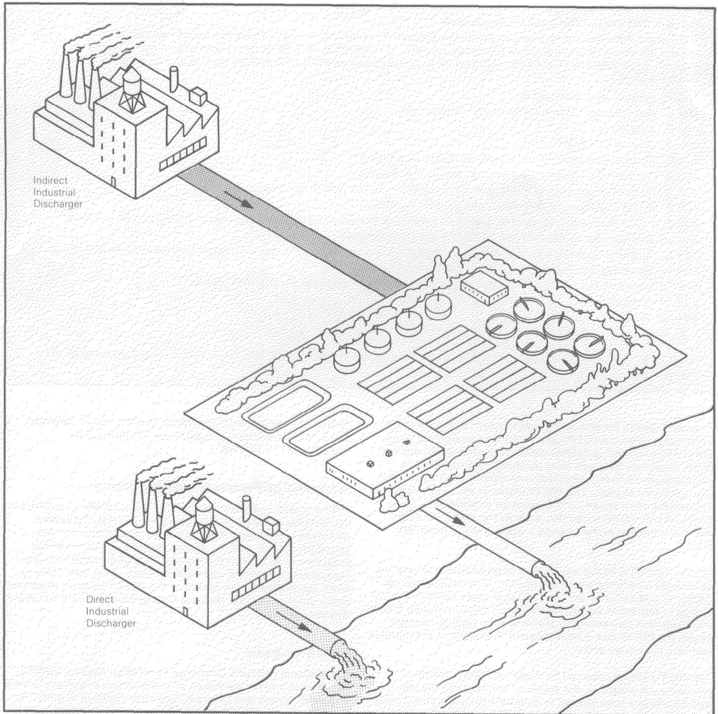
**Figure 8. Direct and Indirect Industrial Dischargers.** Industrial or municipal sewage treatment facilities that discharge their wastewaters directly into rivers, streams, lakes, bays, estuaries, and oceans are referred to as direct dischargers. Industrial facilities that discharge their wastewaters into a municipal sewer system are referred to as indirect dischargers; it is these indirect dischargers that the National Pretreatment Program aims to regulate.
