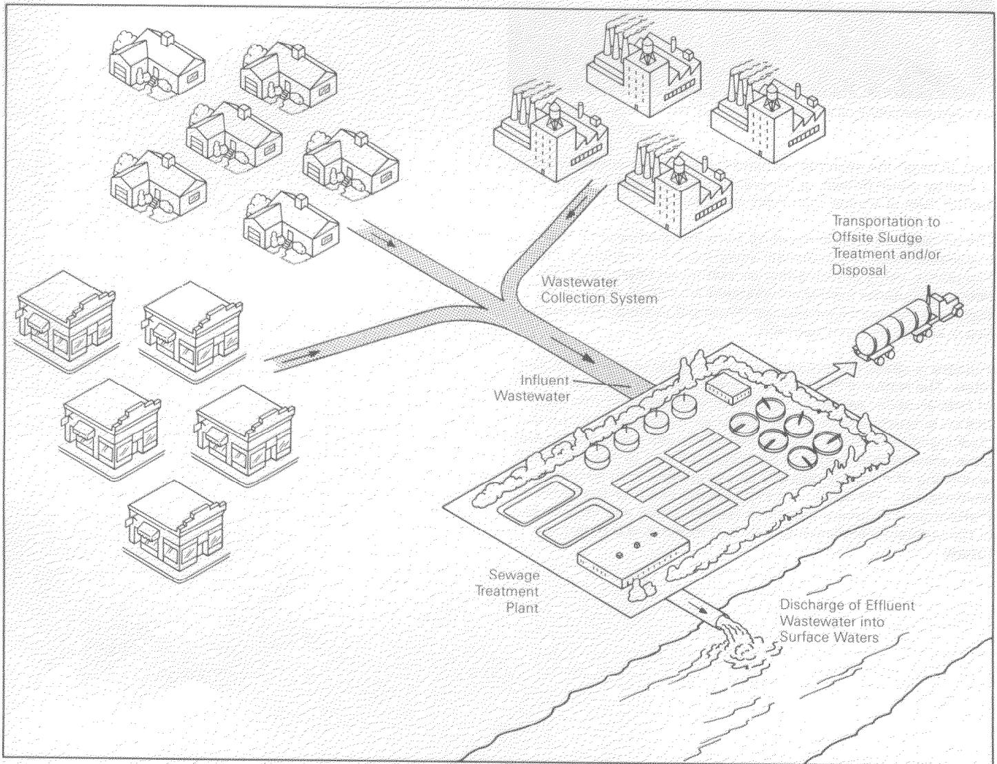
**Figure 1. Wastewater Collection and Treatment.** Industry, households and commercial establishments discharge wastewater into a system of drains, pipes, and pumping stations (a sewage collection system) that channel the flow to the sewage treatment plant. At the plant, the wastewaters are treated and discharged into surface waters. Solids removed from the wastewater during treatment are either disposed of or used productively.
