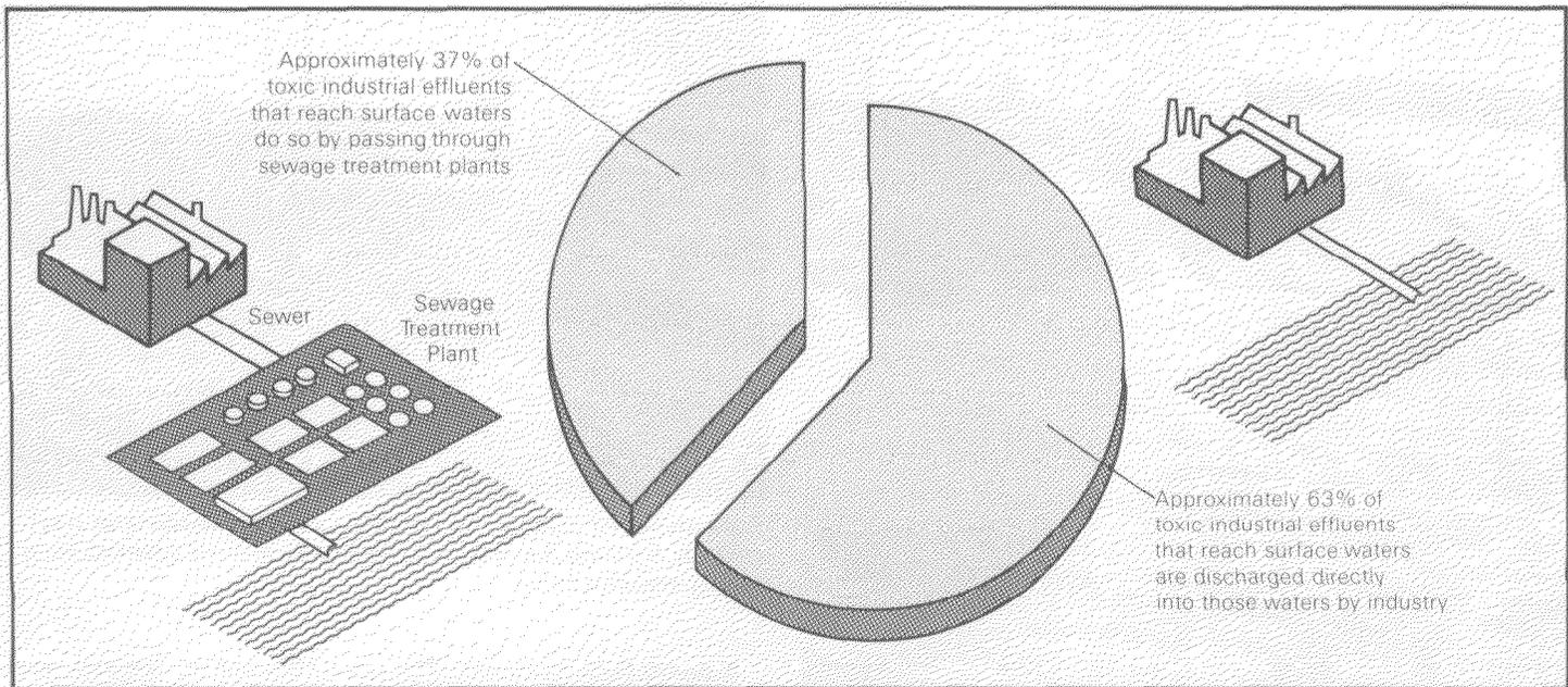
**Figure 4. How Toxic Industrial Effluents Reach Surface Waters.**
