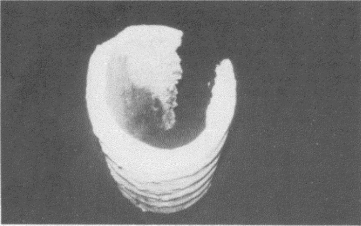
*Concrete sewer corroded by acidic industrial wastewaters.*
