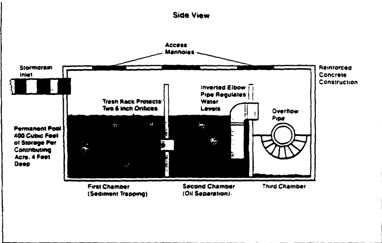
Schematic of a Water Quality Inlet, Rockville Percolating Inlet Design
