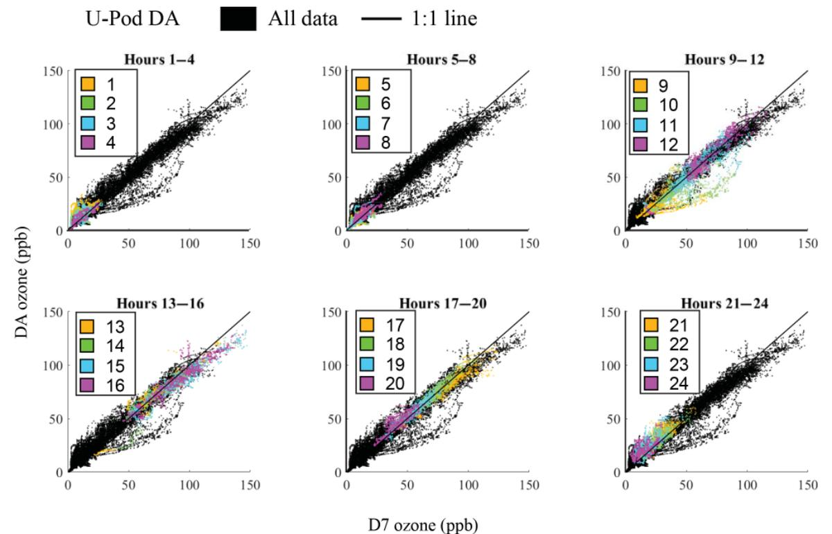
Data from DA, located at Commercial Zone 1, plotted against D7 (Rubidoux). Each scatterplot represents 4 h of the day, with the black data representing the complete deployment dataset (all hours). The black line is a 1 : 1 line.
