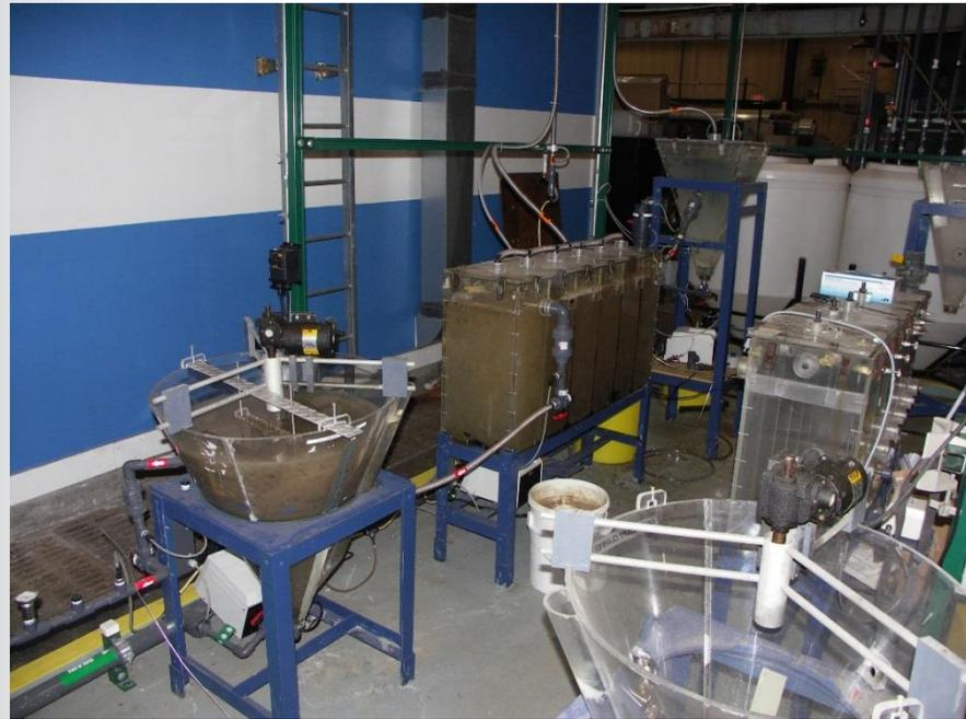
Activated sludge experimental set-up:
