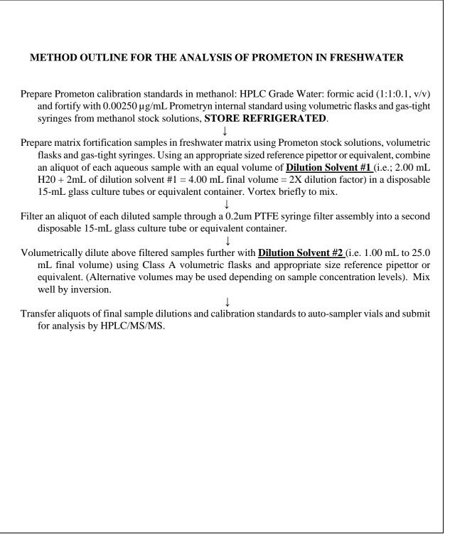
Figure 1. Analytical method outline for the analysis of Prometon in Freshwater.
