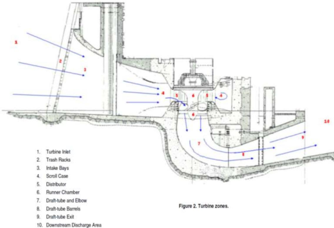
**Figure 2.** Cross-section of hydroelectric generating facility process
