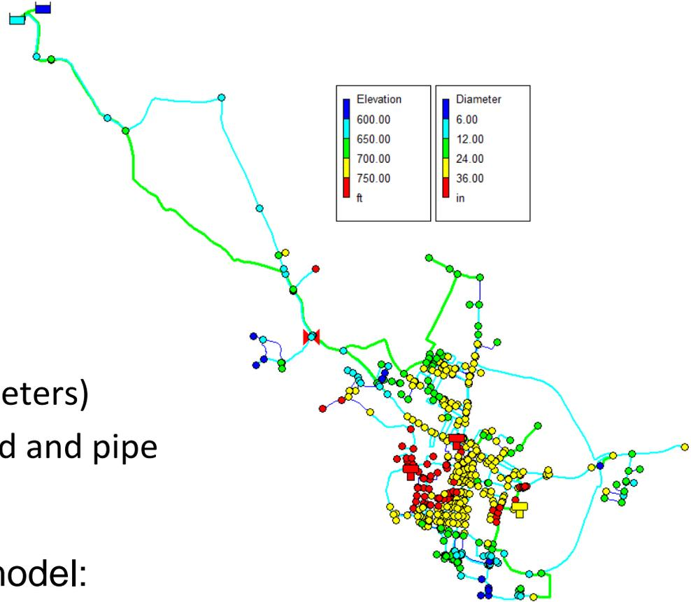
EPANET software uses a network model:
