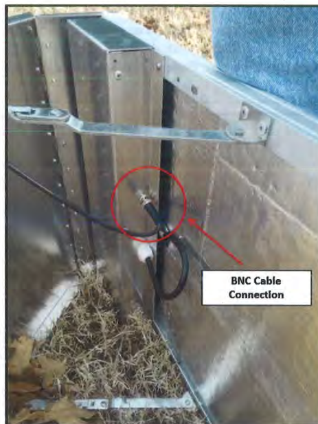
Figure 5. Connecting BNC power cable to solar panel / battery
