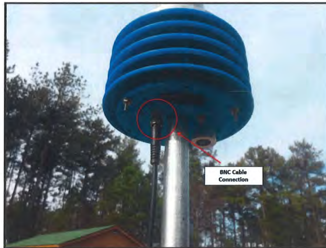
Figure 6. Connecting BNC Power Cable to Sensor Station
