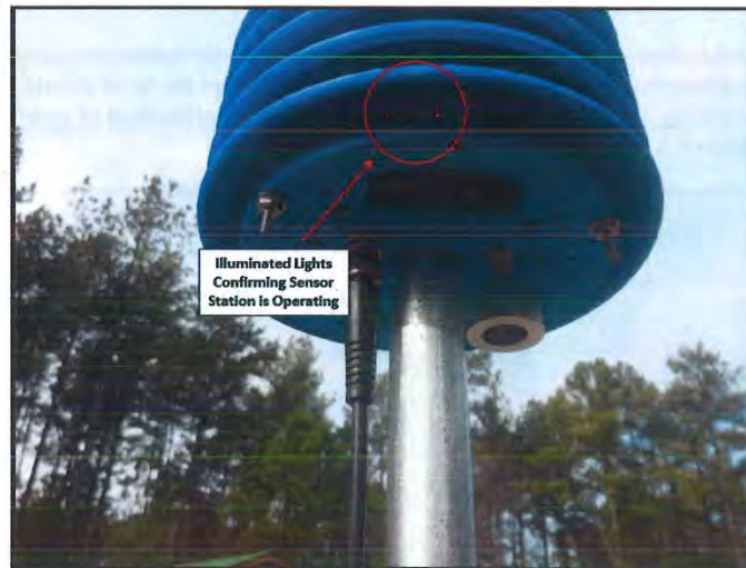
Figure 7. Illuminated lights confirming SPod is operating
