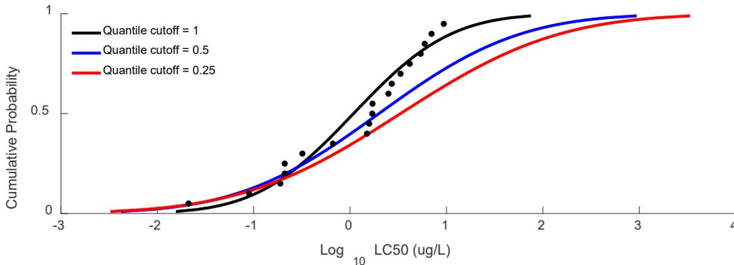
These weighted regressions can accommodate censored data by specifying the lower bound for the censored toxicity endpoints. The quantile cutoff must be lower than the lowest lower bound for censored data. Only linearization can accommodate censored data in this version of the SSD Toolbox.
