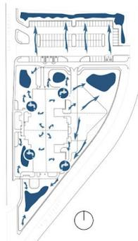
Current retention areas have the potential to support schoolyard vegetation. High incidence of flooding indicates issues with initial grading.
