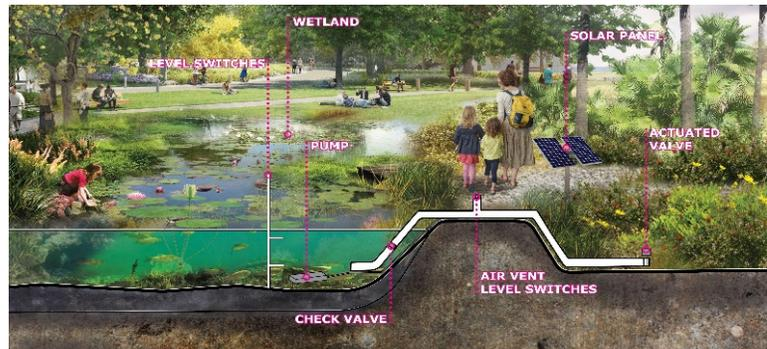
Figure 11. Schematic of our proposed automated and remotely-operated siphon system for water transfer from the lined wetland LW into the tree canopy irrigation network. For our siphon system in action, see <https://www.youtube.com/watch?v=jYkEW8kxsXk>
