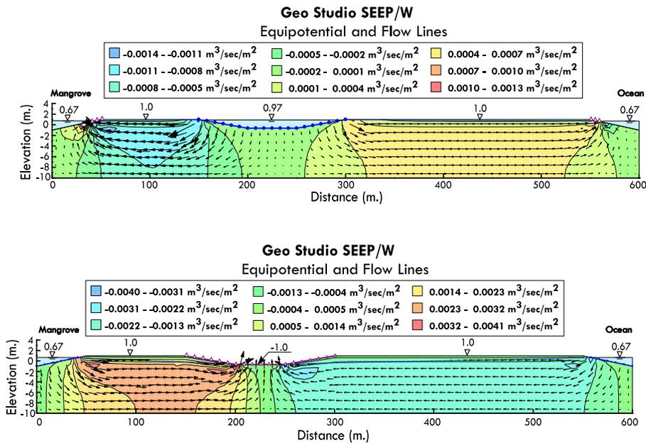
Figure 5. Equipotential and flow line modeling results for the largest existing pond. Black arrows indicate seepage flow directions. **A. Top.** Infiltration (from pond to the Biscayne Bay) and **B. Bottom.** Exfiltration (from Biscayne Bay to the pond).
