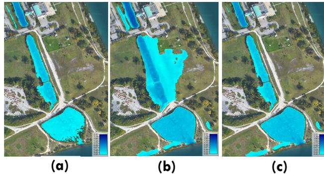
Figure 8. Flood inundation around the south mangrove channel for the 24-hr, 25-year return period for various scenarios. (a) Existing condition (2019) (b) 2050 NOAA sea-level rise projections **without** proposed wetlands (c) 2050 NOAA sea-level rise projections **with** proposed wetlands.
