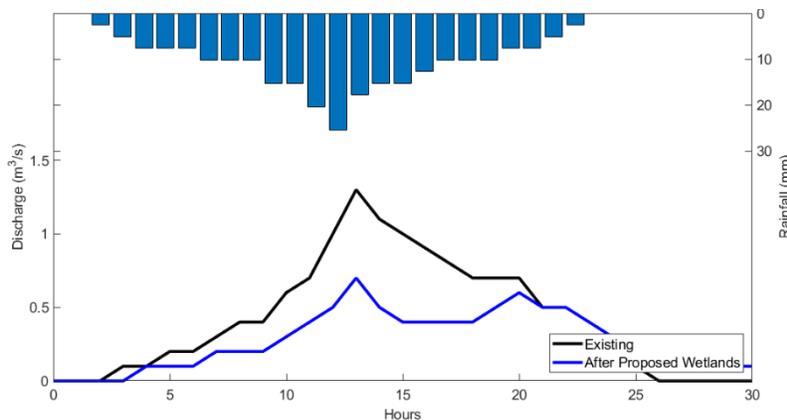
Figure 9. Flow hydrograph at the main channel inlet (point A in Figure 7) for the 2050 NOAA SLR projections with and without the implementation of the proposed wetlands.
