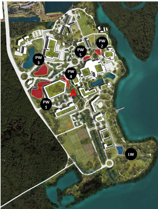
Figure 7. Proposed new wetlands. PW1, PW2, PW3, PW4, PW5 are permeable wetlands for infiltration and pollutant treatment. LW is a lined wetland for stormwater storage for irrigation purposes.
