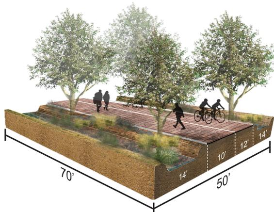
Fig. 10 - Typical 70' x 50' segment of corridor.
