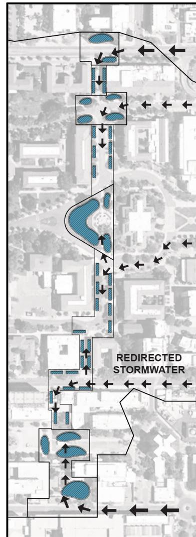
*Fig. 6 - Basin locations and stormwater movement in Phase I segment of western corridor.*
