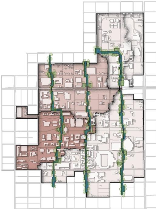
*Fig. 1 - Master plan showing sub-watersheds and location of proposed corridors in green.*
