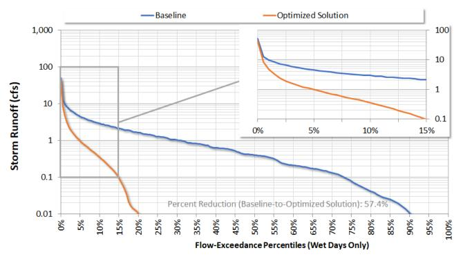
Figure 4-21. Opti-Tool derived flow duration curves for outfall #2
