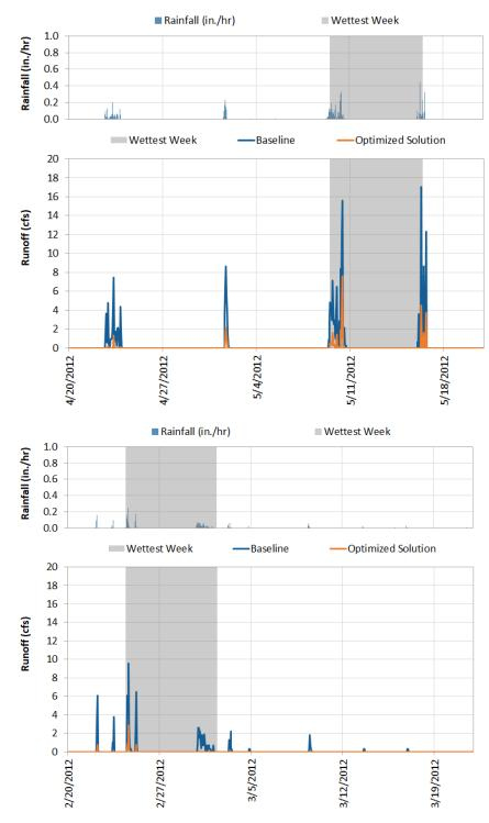
Figure 4-15. Selected periods of rainfall and runoff for outfall #7 during 2012, a year representing an average amount of precipitation for Tisbury, MA. Grey area highlights the wettest week for the period shown.
