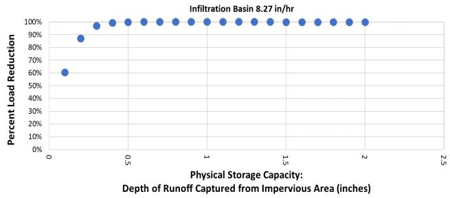
Figure 4-9. Infiltration Basin (8.27 in/hr) performance curve for annual average E. coli load reduction.
