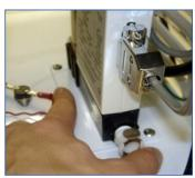
5. Unscrew the (2) Phillips screws on the MFC base plate. This plate will then lift out with the MFC attached. If MFC needs to be replaced/repaired, save the mounting plate separately to avoid accidental discard.
