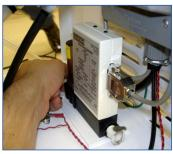
4. Unscrew the (2) flathead screws to loosen and remove the MFC data cable.
