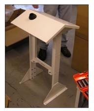
2. Install and tighten all connectors. The roof connector nuts require an 11/32" open end wrench to access the studs at the peak.
