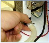
3. Remove the host that connects to the rear of the MFC (and runs to the pump inlet).
