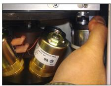
3. You can now use the large wheel located above the solenoid manifold to manually raise and lower the Solenoid Manifold.
