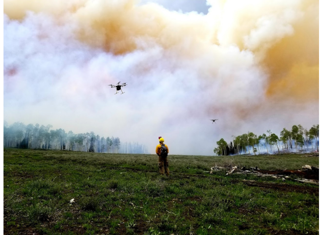
sUAS-based emission sampling during the Fire and Smoke Modeling Evaluation Experiment in Fishlake National Forest, Utah, June 2019. Jess Juchter, Desert Research Institute, used by permission.
