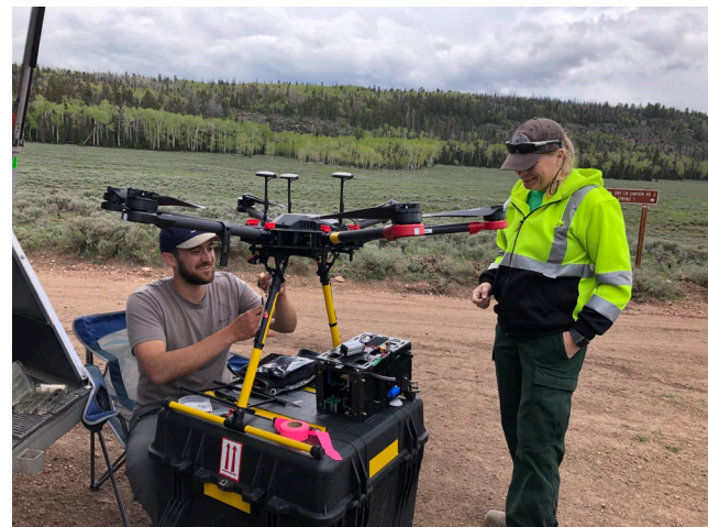
Researchers outfitting sUAS with Kolibri for emission sampling.
