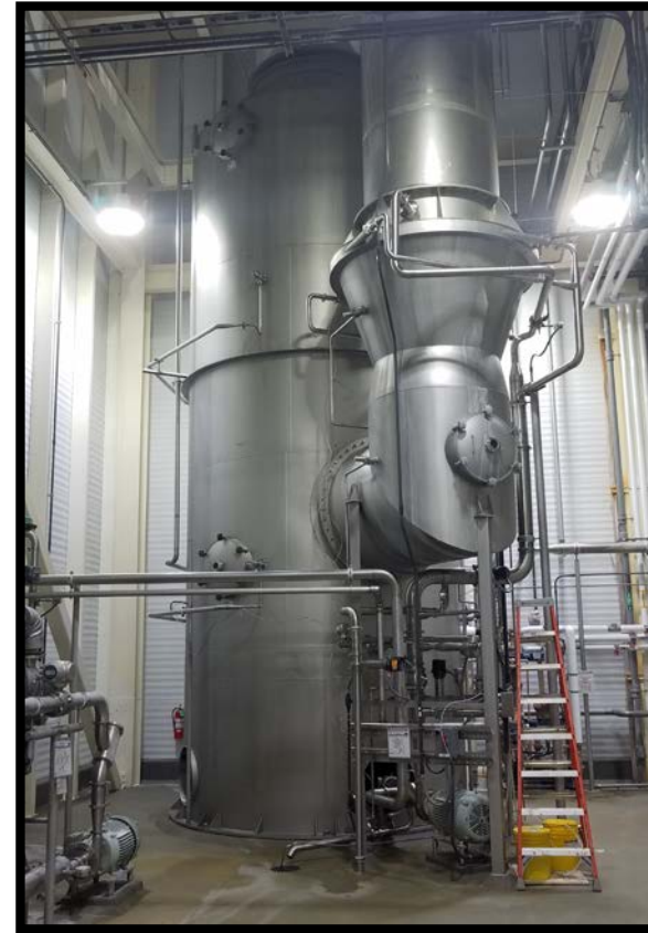
Figure: (Top) Lower portion of scrubber for R3 spray dryer. (R) Water samples were obtained from major assets.
