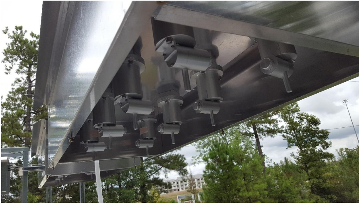
Figure 1. One of four sampling manifolds on the 32-cyclone collocated PE sampler at OAQPS in RTP, NC
