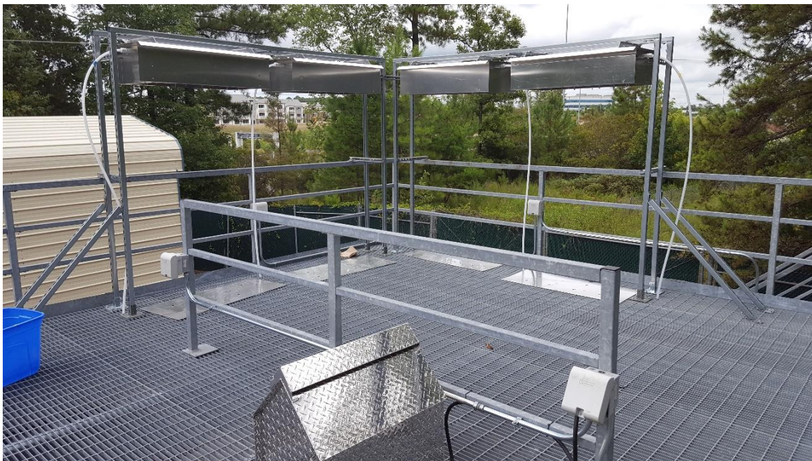
Figure 1. One of four sampling manifolds on the 32-cyclone collocated PE sampler at OAQPS in RTP, NC
