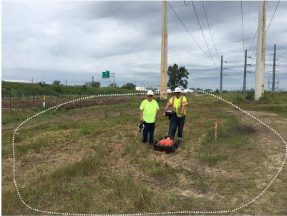
Picture showing where, approximately , the absence of high-amplitude reflections are located.
