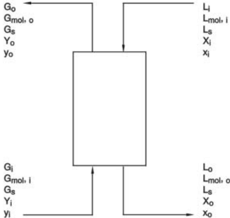
**Figure 1.3:** Schematic Diagram of Countercurrent Packed Bed Operation
