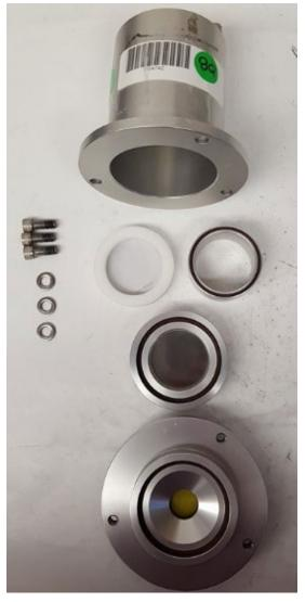
Figure 16. Teflon SASS Exploded View
