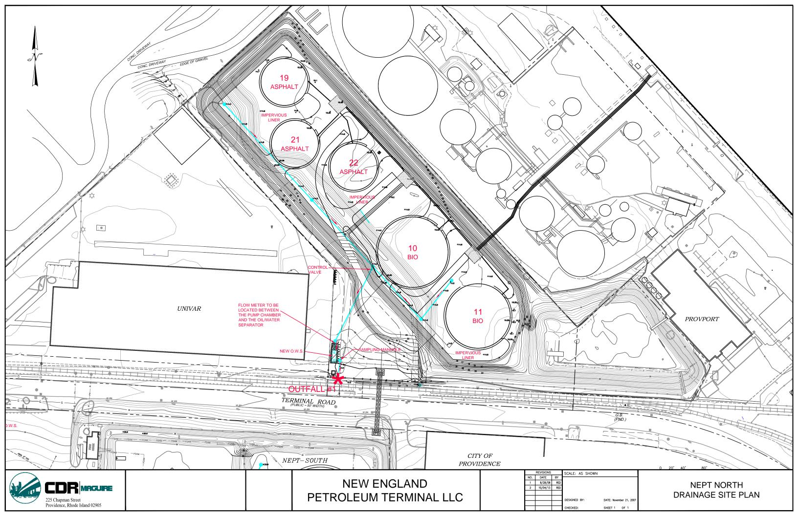
New England Petroleum Terminal, LLC – Northern Terminal HYDROSTATIC TEST WATER LINE FLOW DIAGRAM
