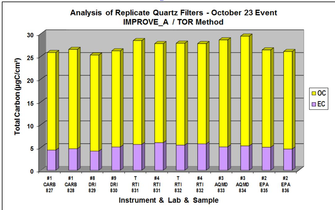
Figure 10 shows results from replicates that were created on October 23, and figure 11 shows the results from replicates created on April 25. The bar segments show the OC and EC components of the total carbon but do not show the more detailed fractions. Notice that each filter submitted to RTI was analyzed more than once using different instruments.
