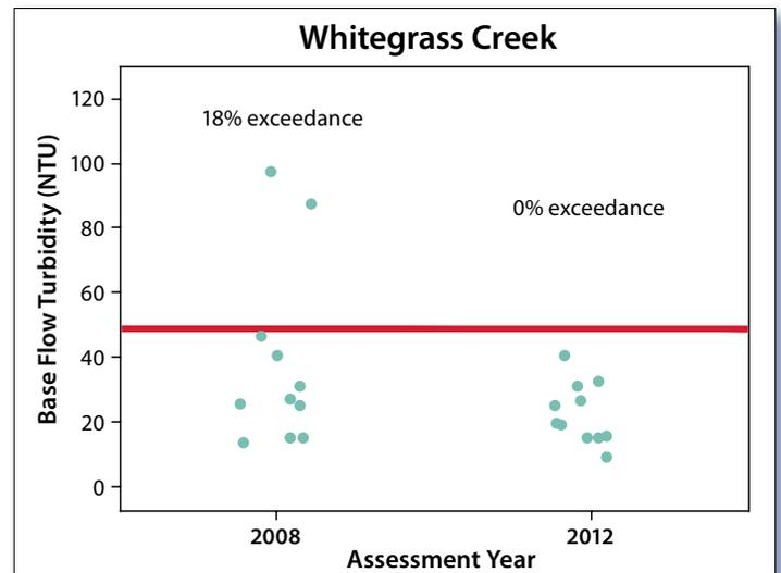
Figure 2. Monitoring data indicate that base flow turbidity levels in Whitegrass Creek have declined.
