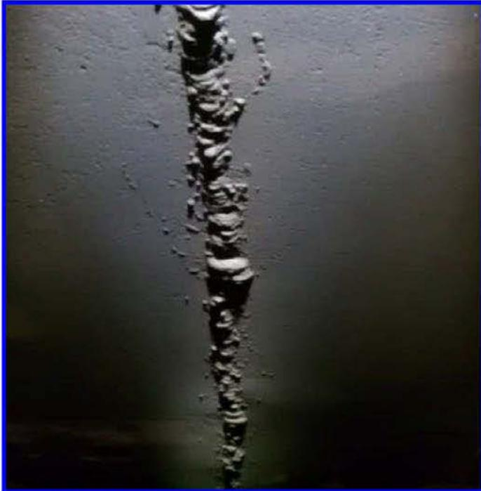
Length of weld with extensive weld spatter
