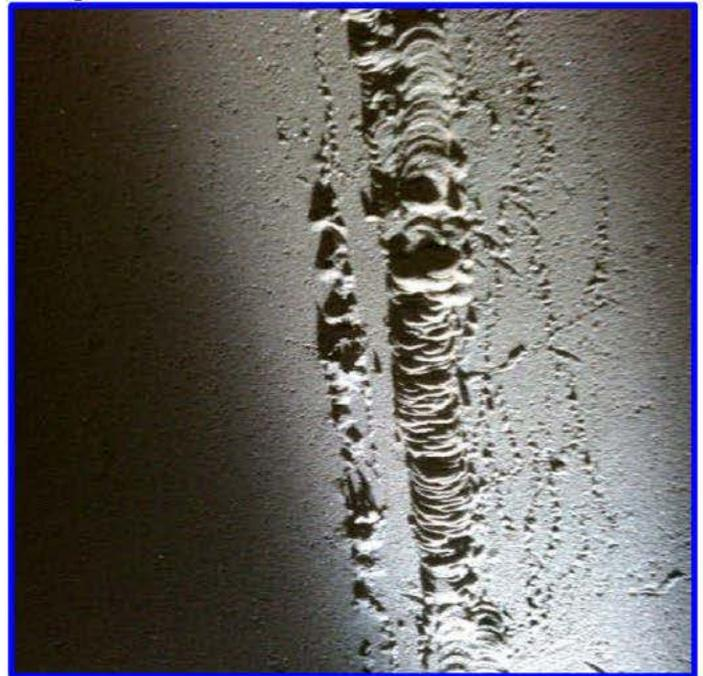
Length of weld with extensive weld spatter
