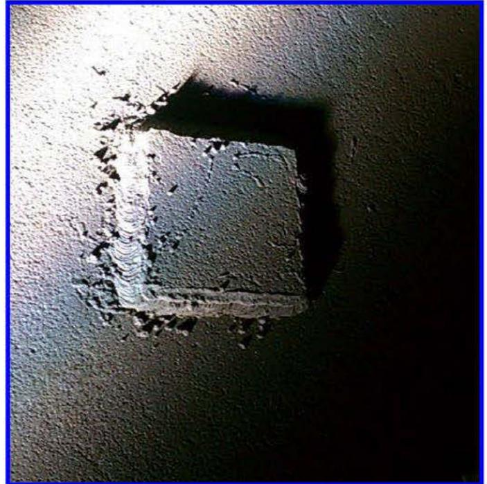
4"X4" welded plate with extensive weld spatter
