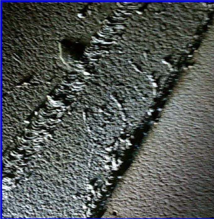
Length of horizontal weld with extensive weld spatter
