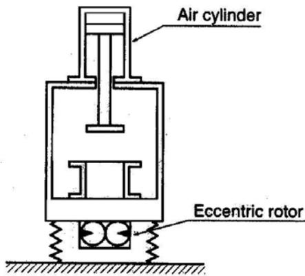
**Figure 2-5. Vibrating Press**
