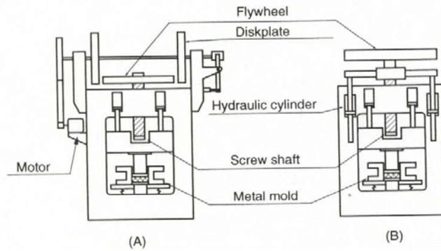
**Figure 2-4. Friction Press (A), and Hydraulic Screw Press (B)**
