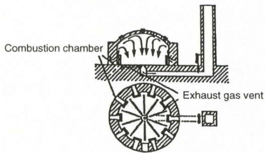
**Figure 2-8. Round Kiln with Downdraft System**
