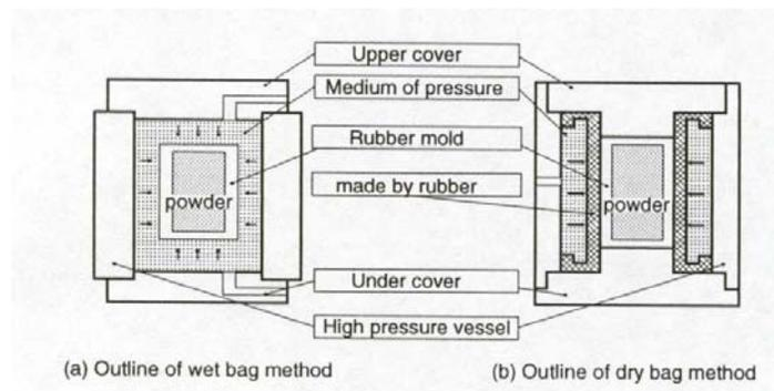
**Figure 2-6. Cross Section of CIP**
