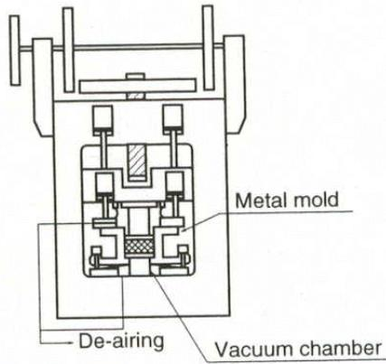
**Figure 2-3. Vacuum Press (Friction, Hydraulic Press)**
