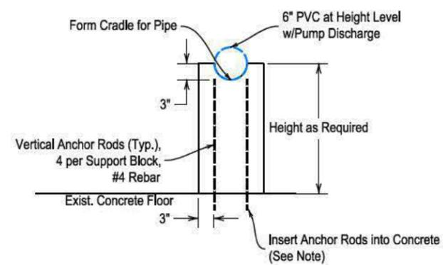
12"x6" Cast-in-Place Concrete Support Detail
