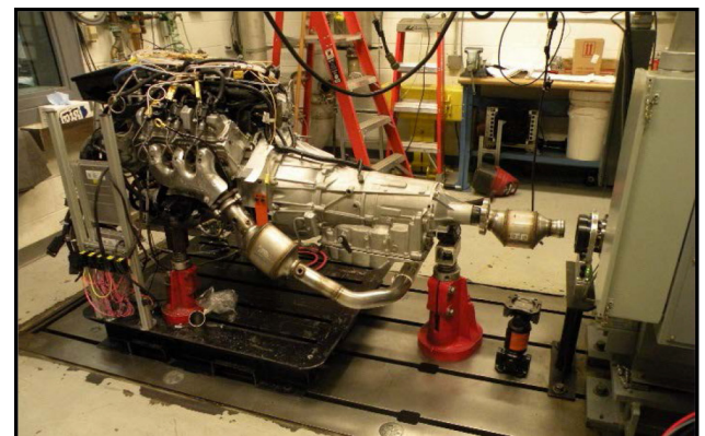
Figure 4. Final Engine and Transmission Test Cell Installation
