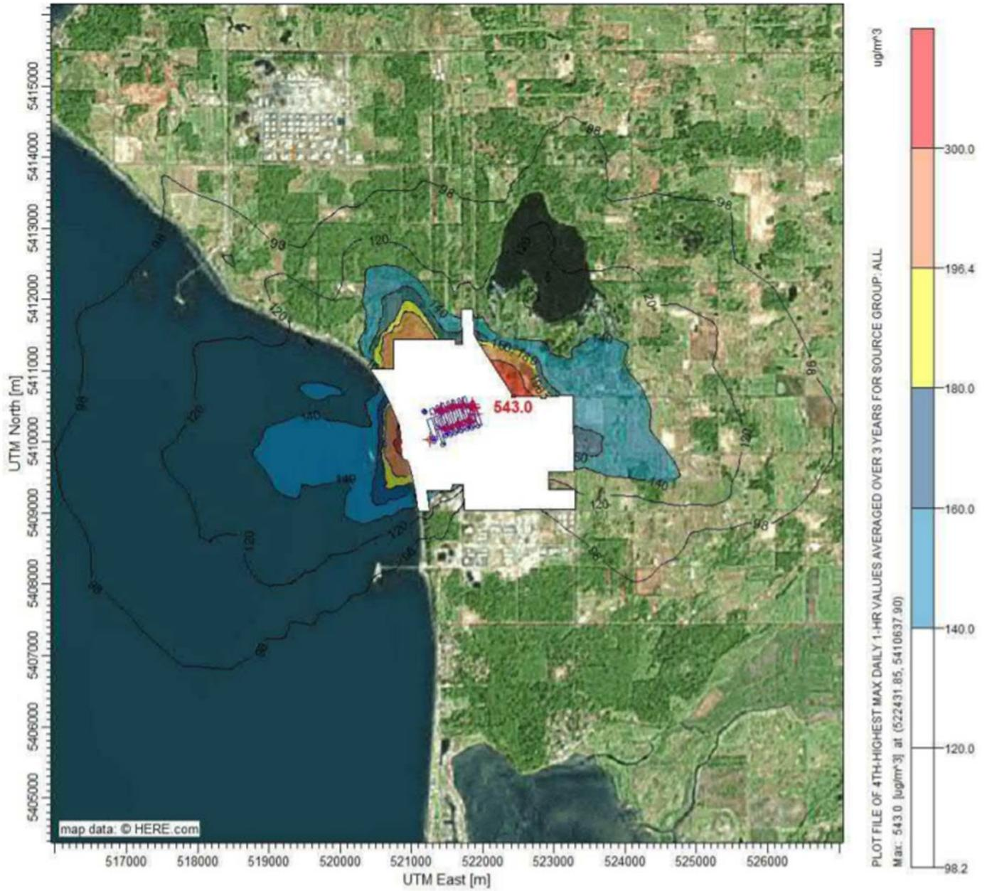
**Figure 11: Predicted 99<sup>th</sup> Percentile Daily Maximum 1-Hour SO<sub>2</sub> Concentrations Averaged Over Three Years for the Area of Analysis for the Whatcom County Area that exceeded the NAAQS (red: violates, green: does not violate) (developed using Google Earth from Google, LLC)**
