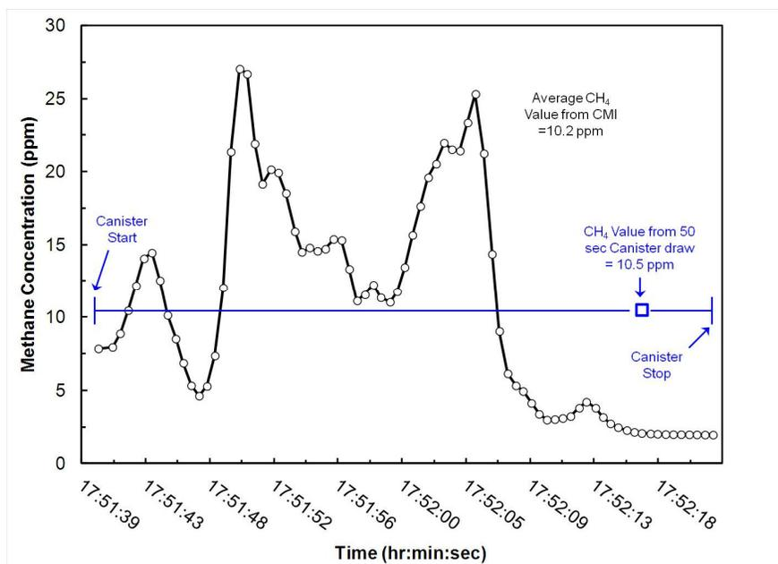
Figure 9-3. Example comparison of CMI and canister data
