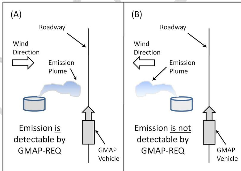
**Figure 2-2. Illustration of limitations of near-source measurements:**
