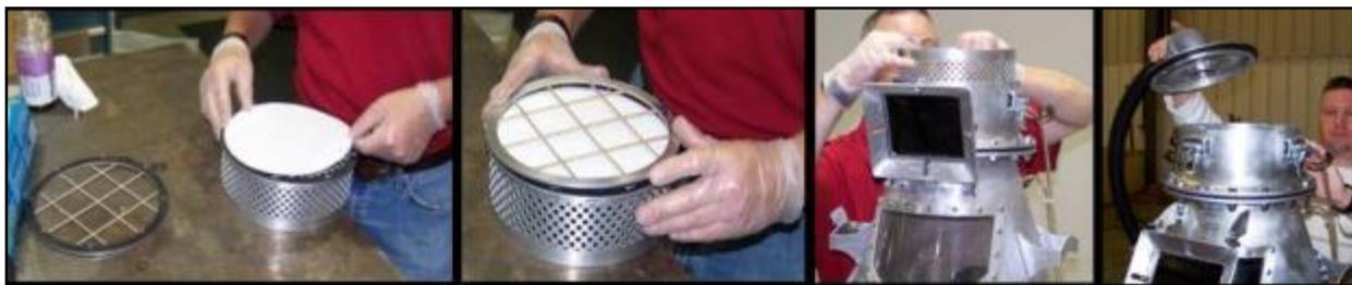
**Figure 7. Placing Filter in Weld Fume Chamber**
