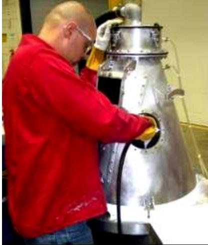
**Figure 8. Welding Inside Weld Fume Chamber**
