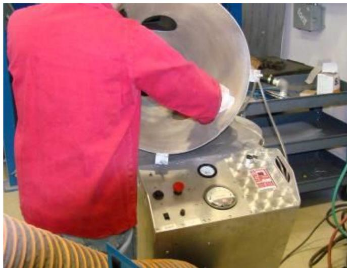
**Figure 14. Cleaning the Chamber between runs**
