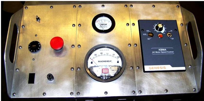
**Figure 2. Control Panel with Gauges**
